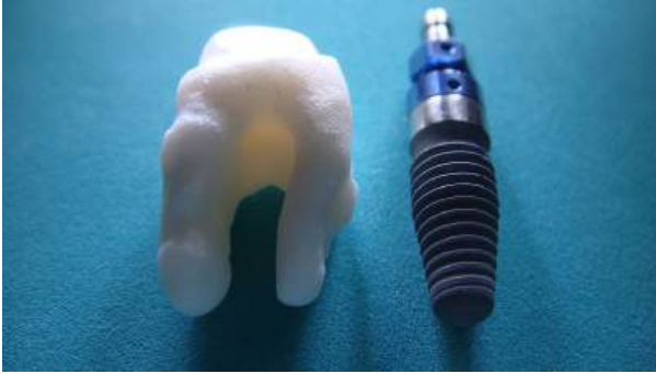
Figure 11.27: Ceramic root analog implant (RAI) compared to a traditional titanium screw-type implant. Image credit: “Own work” by Logicwhattelse is licensed under CC BY-SA 4.0
