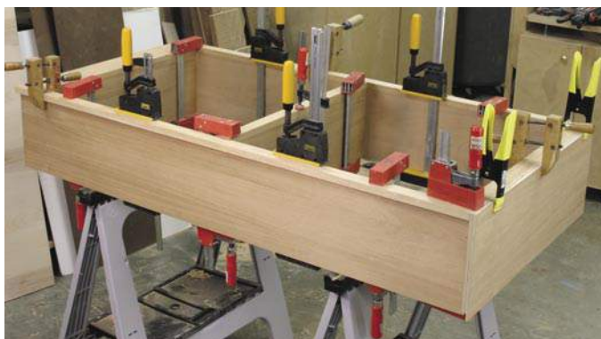
It might take every clamp you own, plus a few borrowed from a neighbor, to attach the face frame. It's worth the effort to get it lined up perfectly without leaving nail holes to be filled.
