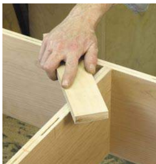
Before attaching the face frame, sand the front edges flush with a flat sanding block. I used a cloth-backed sanding belt glued to plywood.
