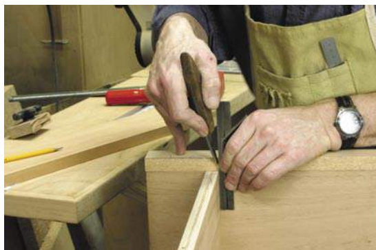
With the stiles clamped to the assembled box, I mark both the length and the exact location of the rails directly. This eliminates errors due to measuring or using undersized plywood.
