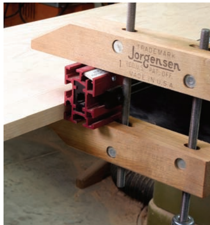
More jigs. Again faced with secure workholding problems at the table saw, I used a handscrew attached to the sliding table to support one end, and a stepoff block at the other to safely locate the groove for the bottom fixed shelf.
