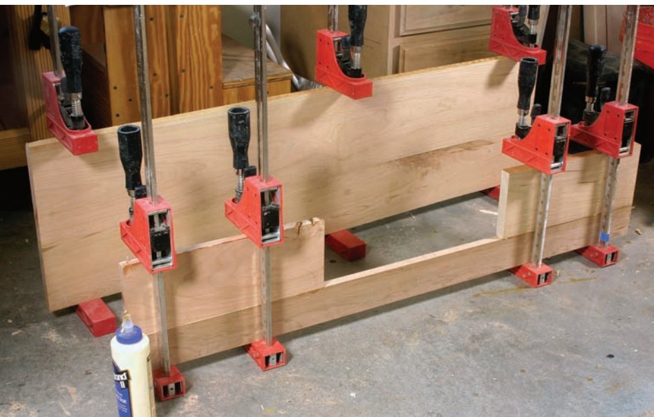
Scabby feet. Because I had very little extra stock, and not enough with matching grain to glue up a solid panel for the curved bottom rail, I had to scab on the foot piece at either end.
