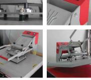
RTC 01 Model Iron + Aluminium **Material Touch Screen Control Panel** Voltage 220 V 6000 W **Power Max Temperature** 250 °C Degree 80 X 100 cm **Press Area Gross Weight** 200 Kg 170 Kg **Net Weight Dimension** 105 x 105 x 63 cm 105 x 105 x 138 cm with stand
