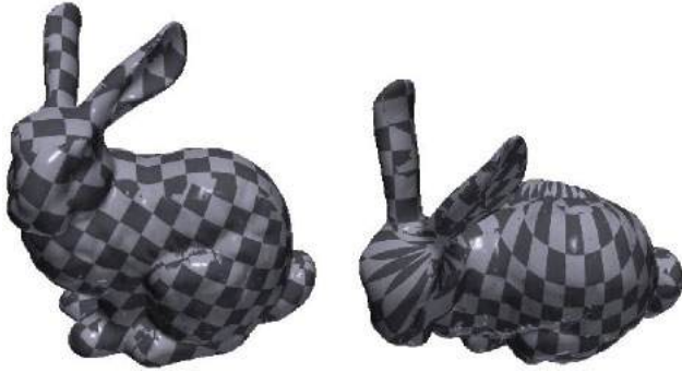
Reparameterized texture using Low Distortion (left) and Fewer Seams (right)
