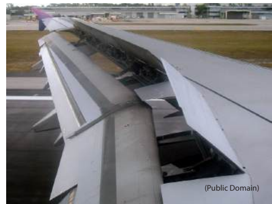
Img. 1 Ground spoilers on an Airbus 320 aircraft
