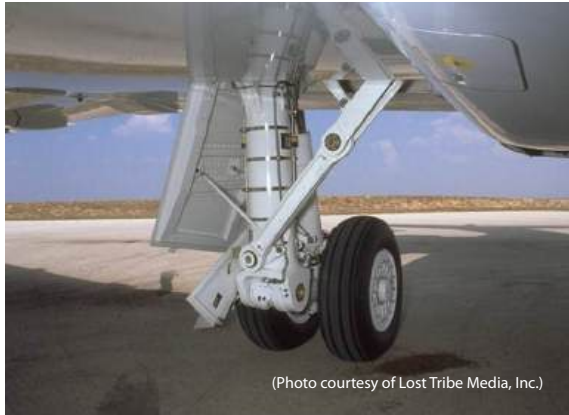
Img. 3 Trailing link landing gear
