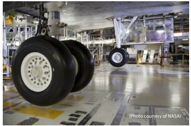
Img. 2 The straight leg landing gear of the Space Shuttle Atlantis
