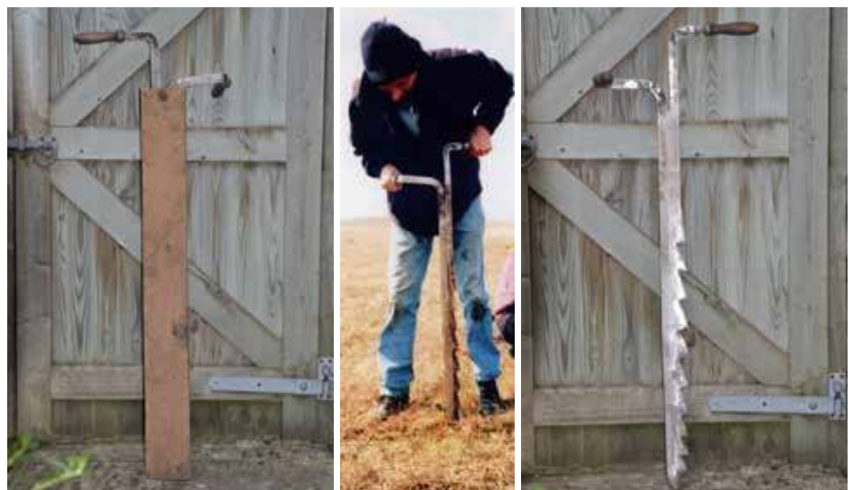
Figure 1: Stainless-steel peat-cutter, showing safety-sheath (left) and field use (center); its sharp edge (right) ensures a clean cut, and minimal environmental damage.
