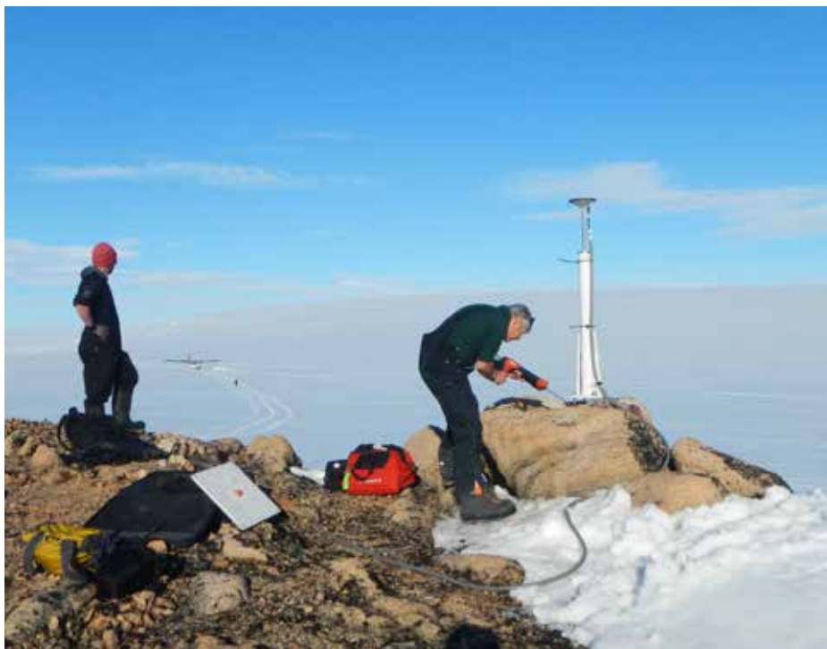
Figure 1: Erik Kendrick (right) installing the GPS monument at Gould Knoll (GLDK) on Thurston Island in the Amundsen Sea. Jeff Amantea (left) looks towards the Twin Otter and broadband seismic station that is part of the POLENET/A-NET project ( polenet.org ) (photo credit: Terry Wilson).
