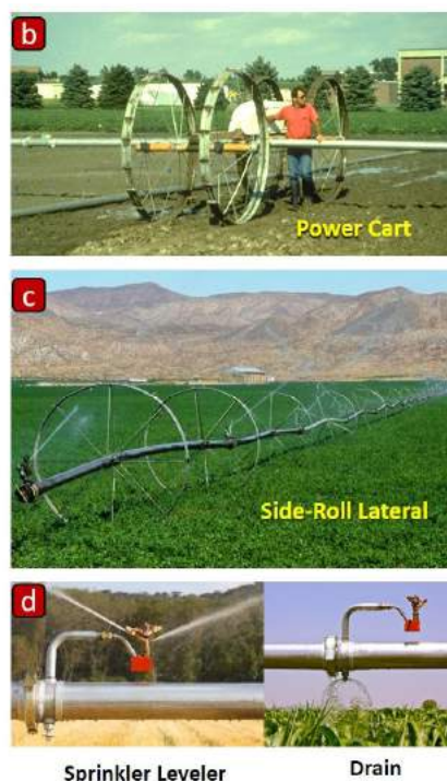
Figure 12.4. Side-roll sprinkler system and components. (The plan view shown in drawing a is adapted from Turner and Anderson, 1980. Picture c is courtesy of Rain for Rent and picture d is courtesy of Wade Rain, Inc.).
