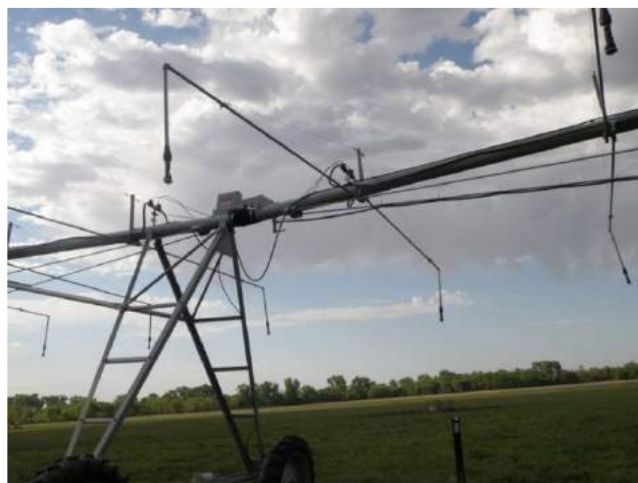
Figure 13.14. Boom backs used to increase wetted diameter for center pivot or lateral move irrigation systems (from Martin et al., 2017).
