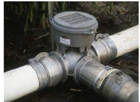
Figure 10.19. Tee-type surge irrigation valve.
