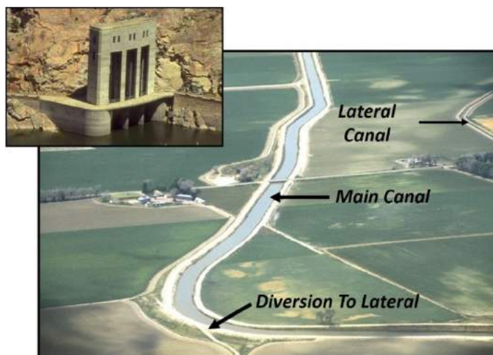
Figure 9.9. Canal delivery system in western Nebraska, which delivers water from Seminoe Dam (inset).
