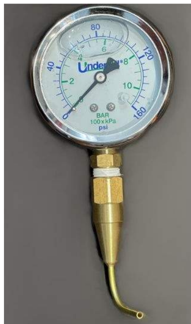
Figure 12.9. Pressure gauge connected to a pitot tube to measure nozzle pressure.
