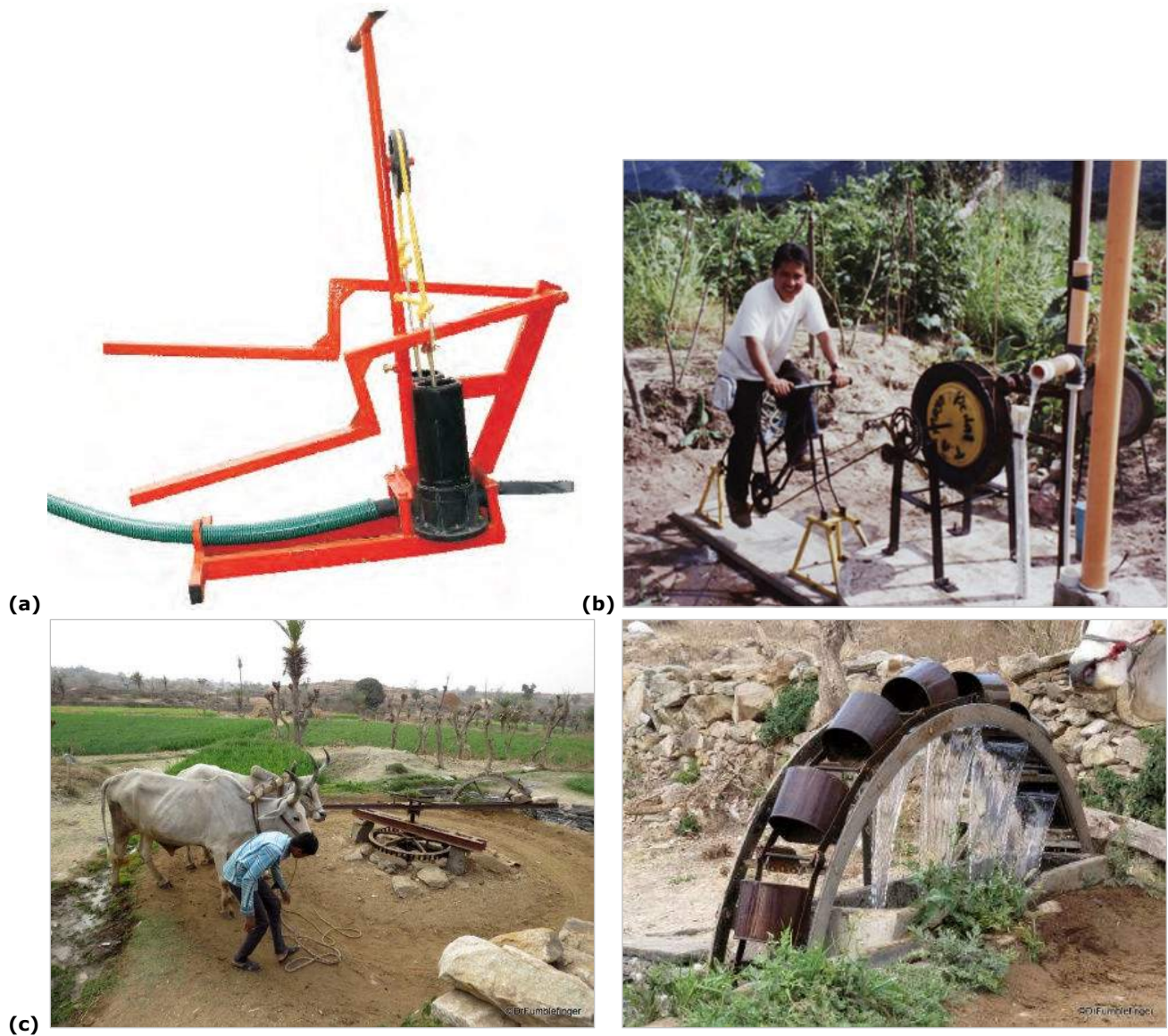
Figure 9.4. Systems for accessing water from shallow aquifers: (a) treadle pump (photo courtesy of iDE, International Development Enterprises); (b) pedal pump (photo courtesy of Maya Pedal Guatemala), and (c) a water wheel in Rajasthan, India (photo courtesy of Carl Anders).
