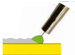
Incorrect. Arc length too long. Arc becomes too wide, giving insufficient penetration and a risk of slag traps. Also a risk of burnback to the contact tip. This may be caused by the arc voltage being too high, the wire feed speed too low or the stick-out being too short.
