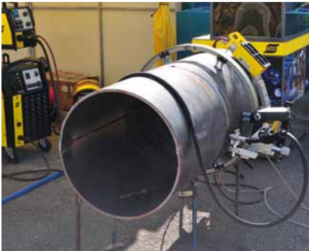
ESAB Railtrac Orbital for circumferential joints.
