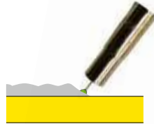
Incorrect. Arc length too short. Wire dips into weld pool (stubbing) caused by too low an arc voltage, too high a wire speed or too long a stick-out.
