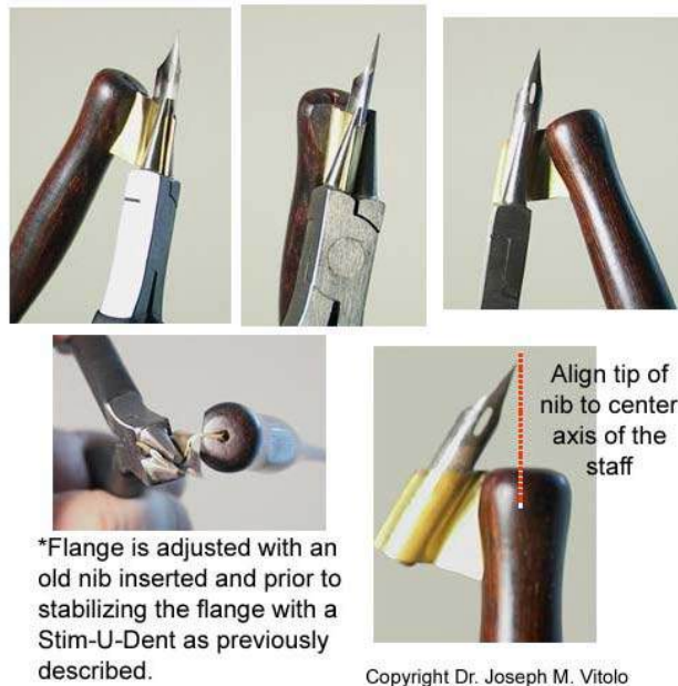
Figure 4. Adjusting the flange before fixation
