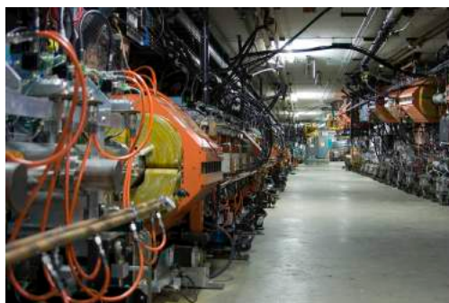
FIGURE 22.24 The Fermilab facility in Illinois has a large particle accelerator (the most powerful in the world until 2008) that employs magnetic fields (magnets seen here in orange) to contain and direct its beam. This and other accelerators have been in use for several decades and have allowed us to discover some of the laws underlying all matter. (credit: ammcgrim, Flickr)
