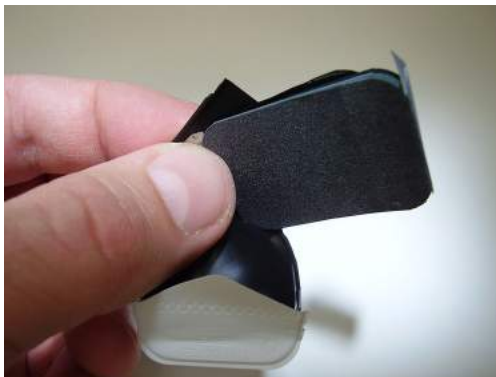
FIGURE 31.7 Film badges contain film similar to that used in this dental x-ray film and is sandwiched between various absorbers to determine the penetrating ability of the radiation as well as the amount. (credit: Werneuchen, Wikimedia Commons)
