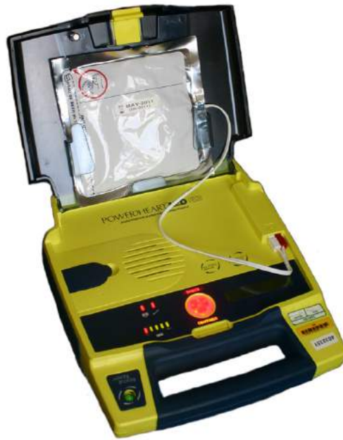
FIGURE 19.23 Automated external defibrillators are found in many public places. These portable units provide verbal instructions for use in the important first few minutes for a person suffering a cardiac attack. (credit: Owain Davies, Wikimedia Commons)
