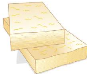
FIGURE 14.16 The fiberglass batt is used for insulation of walls and ceilings to prevent heat transfer between the inside of the building and the outside environment.
