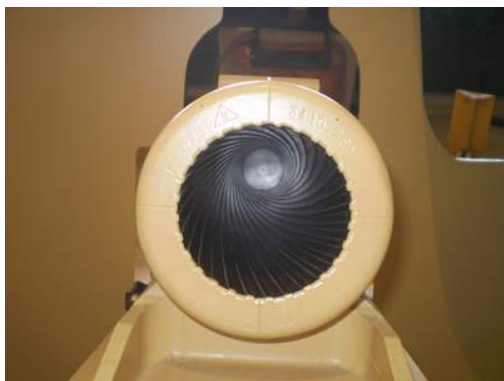
FIGURE 10.34 The image shows a view down the barrel of a cannon, emphasizing its rifling. Rifling in the barrel of a canon causes the projectile to spin just as is the case for rifles (hence the name for the grooves in the barrel). (credit: Elsie esq., Flickr)
