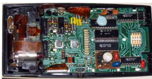
FIGURE 19.22 Energy stored in the large capacitor is used to preserve the memory of an electronic calculator when its batteries are charged. (credit: Kucharek, Wikimedia Commons)
