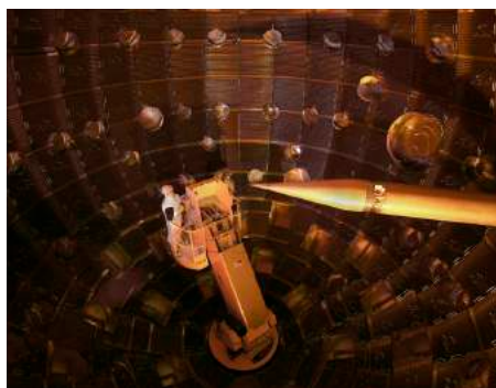
FIGURE 30.39 This system of lasers at Lawrence Livermore Laboratory is used to ignite nuclear fusion. A tremendous burst of energy is focused on a small fuel pellet, which is imploded to the high density and temperature needed to make the fusion reaction proceed. (credit: Lawrence Livermore National Laboratory, Lawrence Livermore National Security, LLC, and the Department of Energy)
