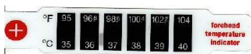
FIGURE 13.4 Each of the six squares on this plastic (liquid crystal) thermometer contains a film of a different heat-sensitive liquid crystal material. Below 95°F, all six squares are black. When the plastic thermometer is exposed to temperature that increases to 95°F, the first liquid crystal square changes color. When the temperature increases above 96.8°F the second liquid crystal square also changes color, and so forth. (credit: Arkrishna, Wikimedia Commons)
