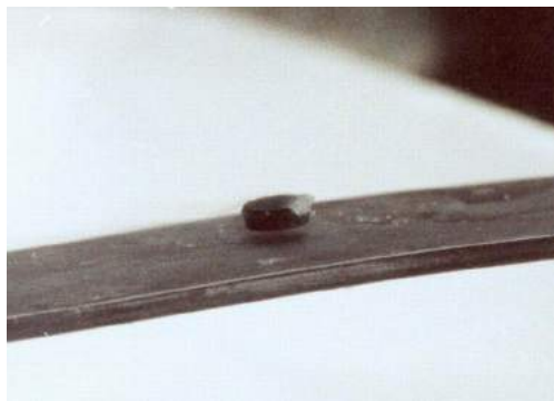
FIGURE 34.24 One characteristic of a superconductor is that it excludes magnetic flux and, thus, repels other magnets. The small magnet levitated above a high-temperature superconductor, which is cooled by liquid nitrogen, gives evidence that the material is superconducting. When the material warms and becomes conducting, magnetic flux can penetrate it, and the magnet will rest upon it. (credit: Saperaud)
