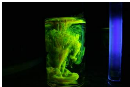
FIGURE 30.31 Here, fluorescent powder is added to a beaker of water. The mixture gives off a bright glow under ultraviolet light. (credit: Bricksnite, Wikimedia Commons)
