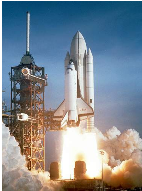
FIGURE 8.13 The space shuttle had a number of reusable parts. Solid fuel boosters on either side were recovered and refueled after each flight, and the entire orbiter returned to Earth for use in subsequent flights. The large liquid fuel tank was expended. The space shuttle was a complex assemblage of technologies, employing both solid and liquid fuel and pioneering ceramic tiles as reentry heat shields. As a result, it permitted multiple launches as opposed to single-use rockets. (credit: NASA)
