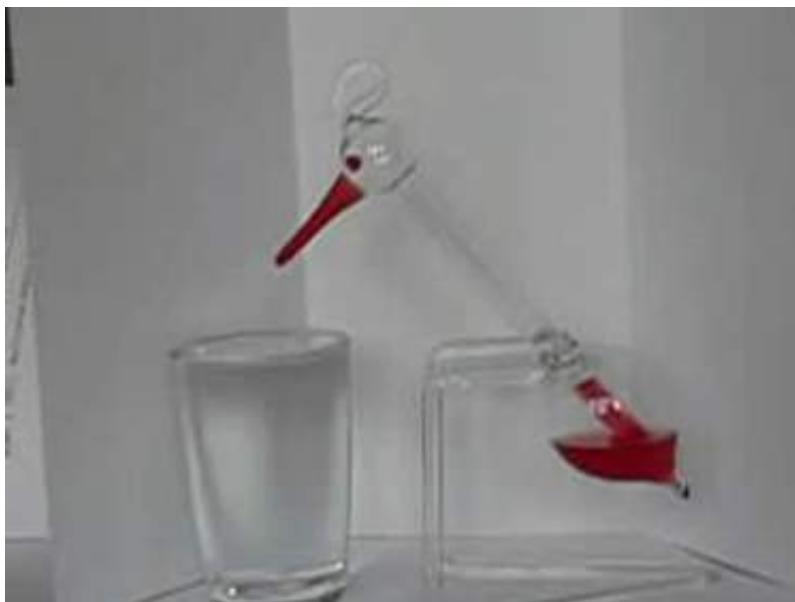
FIGURE 15.20 This novelty toy, known as the drinking bird, is an example of Carnot's engine. It contains methylene chloride (mixed with a dye) in the abdomen, which boils at a very low temperature—about 100°F. To operate, one gets the bird's head wet. As the water evaporates, fluid moves up into the head, causing the bird to become top-heavy and dip forward back into the water. This cools down the methylene chloride in the head, and it moves back into the abdomen, causing the bird to become bottom heavy and tip up. Except for a very small input of energy—the original head-wetting—the bird becomes a perpetual motion machine of sorts. (credit: Arabesk.nl, Wikimedia Commons)
