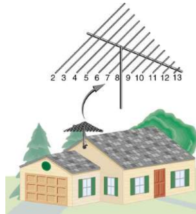
FIGURE 24.26 A television reception antenna has cross wires of various lengths to most efficiently receive different wavelengths.
