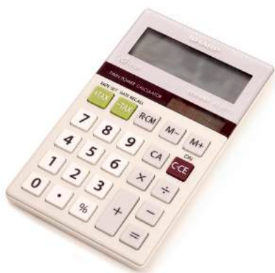
FIGURE 20.36 The strip of solar cells just above the keys of this calculator convert light to electricity to supply its energy needs. (credit: Evan-Amos, Wikimedia Commons)
