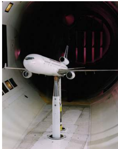
FIGURE 5.8 NASA researchers test a model plane in a wind tunnel. (credit: NASA/Ames)
