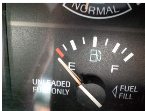
FIGURE 13.13 Because the gas expands more than the gas tank with increasing temperature, you can't drive as many miles on “empty” in the summer as you can in the winter. (credit: Hector Alejandro, Flickr)
