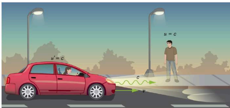
FIGURE 28.15 According to experiment and the second postulate of relativity, light from the car's headlights moves away from the car at speed c and towards the observer on the sidewalk at speed c . Classical velocity addition is not valid.
