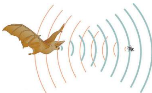
FIGURE 17.9 A bat uses sound echoes to find its way about and to catch prey. The time for the echo to return is directly proportional to the distance.
