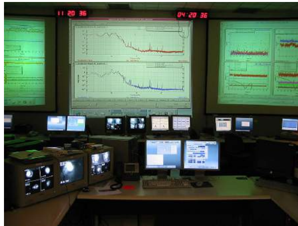
FIGURE 34.15 The control room of the LIGO gravitational wave detector. Gravitational waves will cause extremely small vibrations in a mass in this detector, which will be detected by laser interferometer techniques. Such detection in coincidence with other detectors and with astronomical events, such as supernovas, would provide direct evidence of gravitational waves. (credit: Tobin Fricke)
