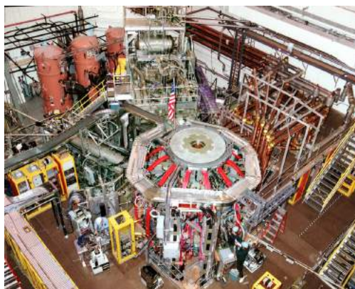
FIGURE 28.20 The National Spherical Torus Experiment (NSTX) has a fusion reactor in which hydrogen isotopes undergo fusion to produce helium. In this process, a relatively small mass of fuel is converted into a large amount of energy. (credit: Princeton Plasma Physics Laboratory)
