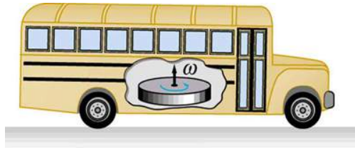
FIGURE 10.15 Experimental vehicles, such as this bus, have been constructed in which rotational kinetic energy is stored in a large flywheel. When the bus goes down a hill, its transmission converts its gravitational potential energy into KE_{\text{rot}} . It can also convert translational kinetic energy, when the bus stops, into KE_{\text{rot}} . The flywheel's energy can then be used to accelerate, to go up another hill, or to keep the bus from slowing down due to friction.
