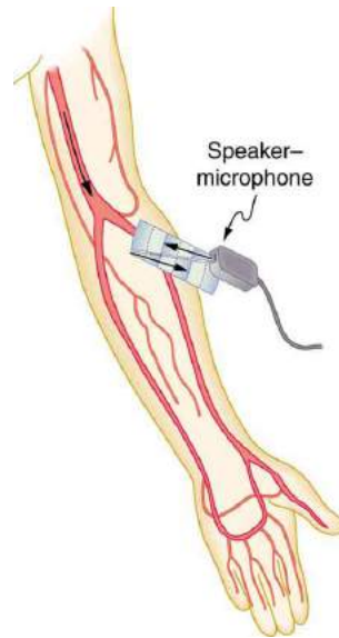
FIGURE 17.46 Ultrasound is partly reflected by blood cells and plasma back toward the speaker-microphone. Because the cells are moving, two Doppler shifts are produced—one for blood as a moving observer, and the other for the reflected sound coming from a moving source. The magnitude of the shift is directly proportional to blood velocity.
