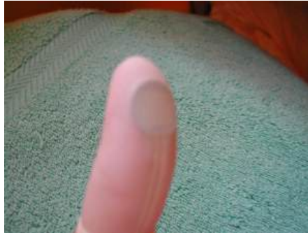
Figure 1.15: Image of large sensor head secured to the medial aspect of the thumb using the thumb section of a latex glove.
