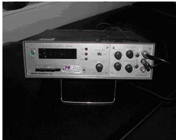
Figure 2.2: Malden Electronics Ltd Digital timer 8816. Used for the Sham TENS (control) procedure. The non-pad ends of the TENS leads were attached to the back of the equipment by crocodile clips to give the impression of functioning equipment.
