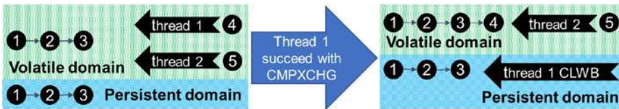
Figure 14-2. Example of a concurrent lock-free insert operation to a singly linked list located in persistent memory
