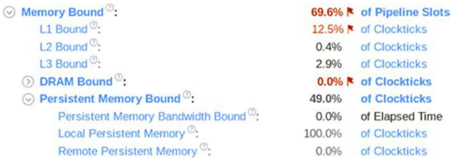
Figure 15-9. VTune Profiler memory analysis of a workload showing a breakdown of CPU cache, DRAM, and persistent memory accesses
