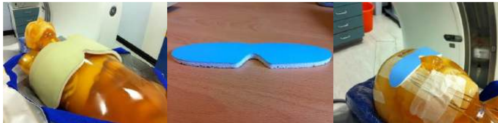
Figure 9.5 Examples of bismuth patient protection shields for breast and thyroid (courtesy Robert Loader)
