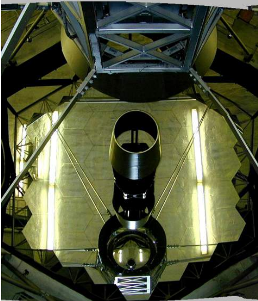
Thirty-Six Eyes Are Better Than One - Figure 3. The mirror of the 10-meter Keck telescope is composed of 36 hexagonal sections. (credit: NASA)
