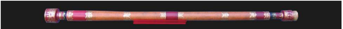
Telescope Used by Galileo - Image 5. The telescope has a wooden tube covered with paper and a lens 26 millimeters across.
