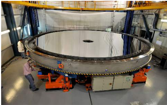
Large Telescope Mirror - Figure 1. This image shows one of the primary mirrors of the European Southern Observatory’s Very Large Telescope, named Yepun, just after it was recoated with aluminum. The mirror is a little over 8 meters in diameter. (credit: ESO/G. Huedepohl)
