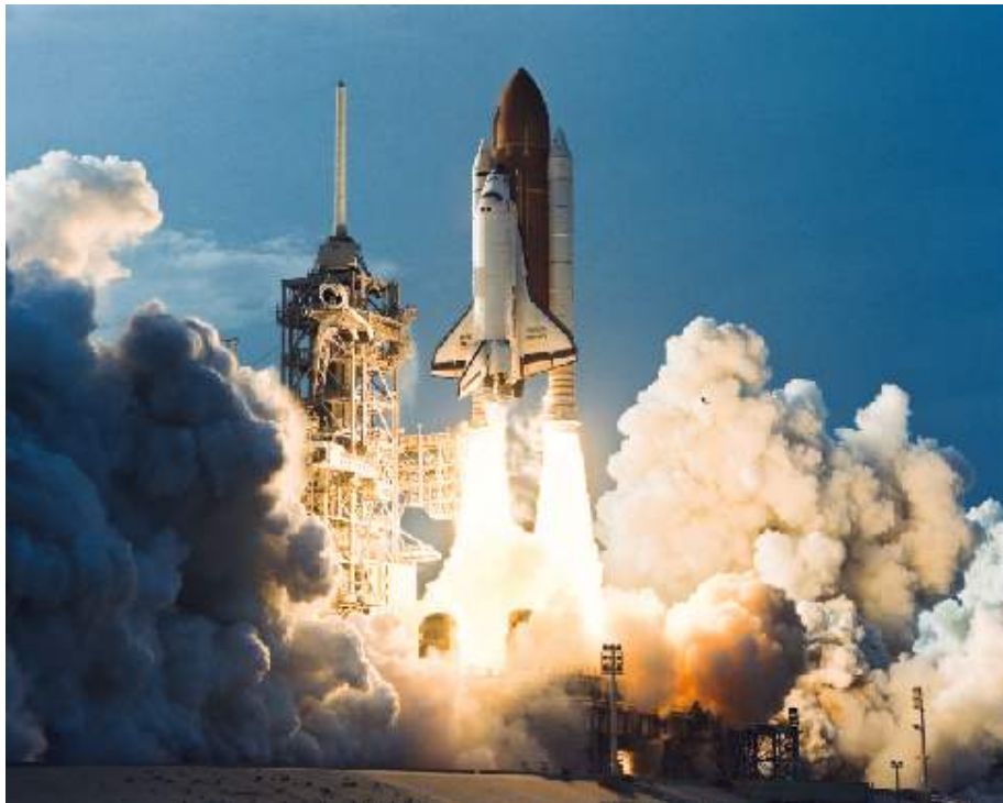
Demonstrating Newton's Third Law - Figure 2. The U.S. Space Shuttle (here launching Discovery), powered by three fuel engines burning liquid oxygen and liquid hydrogen, with two solid fuel boosters, demonstrates Newton's third law. (credit: modification of work by NASA)
