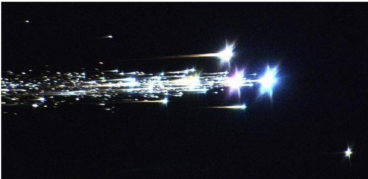
Hayabusa Return - Figure 9. This dramatic image shows the Hayabusa probe breaking up upon reentry. The return capsule, which separated from the main spacecraft and parachuted to the surface, glows at the bottom right. (credit: modification of work by NASA Ames/Jesse Carpenter/Greg Merkes)
