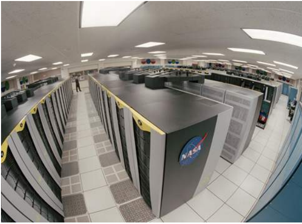
Modern Computing Power - Figure 1. These supercomputers at NASA's Ames Research Center are capable of tracking the motions of more than a million objects under their mutual gravitation. (credit: NASA Ames Research Center/Tom Trower)
