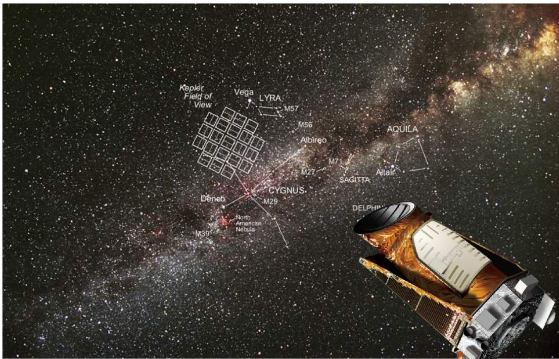
Kepler’s Field of View - Figure 5. The boxes show the region where the Kepler spacecraft cameras took images of over 150,000 stars regularly, to find transiting planets. (credit “field of view”: modification of work by NASA/Kepler mission; credit “spacecraft”: modification of work by NASA/Kepler mission/Wendy Stenzel)
