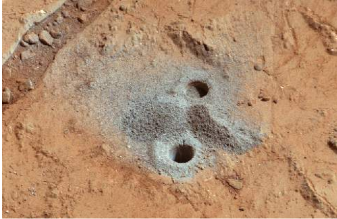
Mudstone - Figure 1. Shown are the first holes drilled by NASA's Curiosity Mars rover into a mudstone, with "fresh" drill-pilings around the holes. Notice the difference in color between the red ancient martian surface and the gray newly exposed rock powder that came from the drill holes. Each drill hole is about 0.6 inch (1.6 cm) in diameter. (credit: modification of work by NASA/JPL-Caltech/MSSS)
