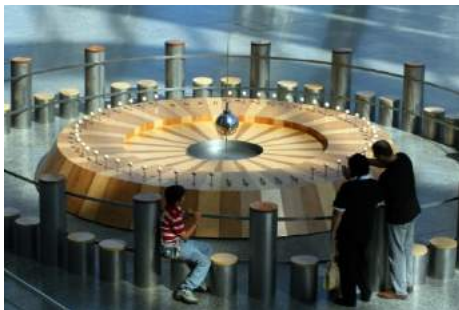
Foucault’s Pendulum - Image 3. As Earth turns, the plane of oscillation of the Foucault pendulum shifts gradually so that over the course of 12 hours, all the targets in the circle at the edge of the wooden platform are knocked over in sequence. (credit: Manuel M. Vicente)
