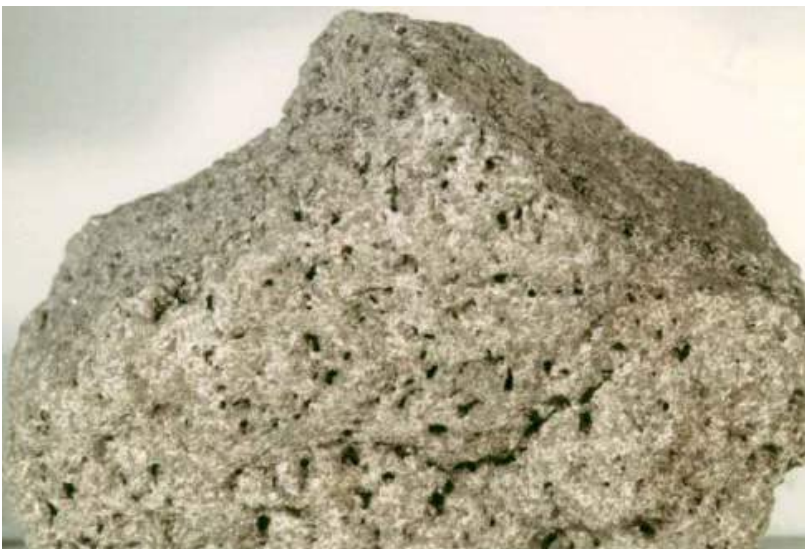
Rock from a Lunar Mare - Figure 5. In this sample of basalt from the mare surface, you can see the holes left by gas bubbles, which are characteristic of rock formed from lava. All lunar rocks are chemically distinct from terrestrial rocks, a fact that has allowed scientists to identify a few lunar samples among the thousands of meteorites that reach Earth. (credit: modification of work by NASA)
