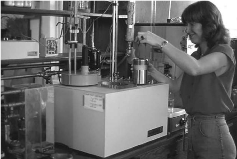
Fig. 7.9. A bomb calorimeter used in the determination of the calorie content of feeds. The bomb (the container in which the feed sample is burned) is in the technician's right hand. The feed sample is put into a cup in her left hand and then inserted into the bomb. (Courtesy of OSU Rabbit Research Center)
