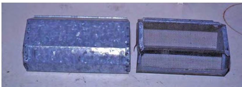
Fig. 4.13. An example of a J feeder, with a mesh bottom to allow fines to sift out of the feed (right) and a feeder with a solid bottom (left). (Courtesy of D.J. Harris)
