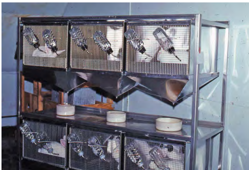
Fig. 7.7. Metabolism cages, which allow separate collection of feces and urine. These are used for such purposes as the measurement of nutrient digestibility. (Courtesy of D.J. Harris)
