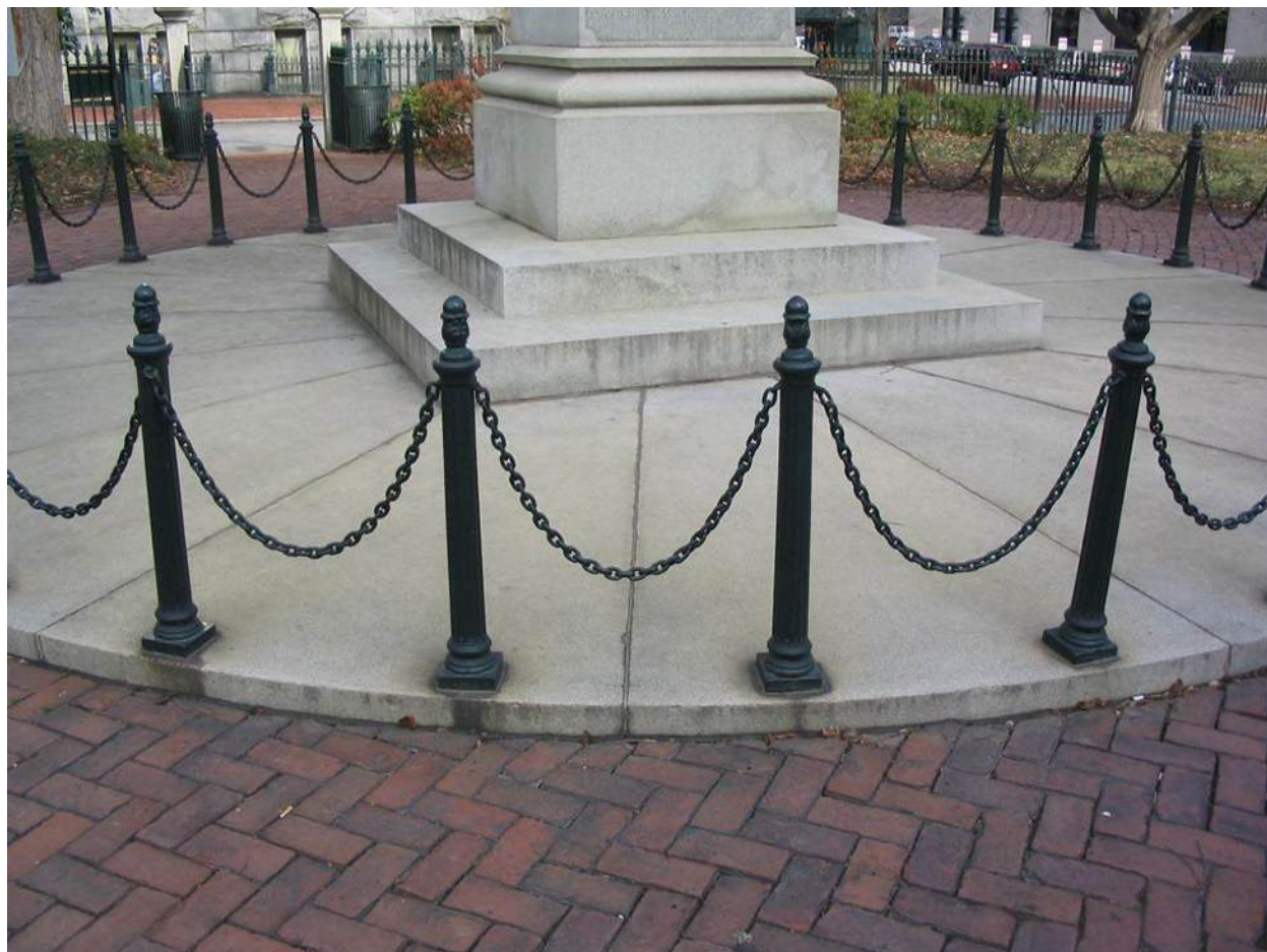
Figure 6.83 Chains between these posts take the shape of a catenary. (credit: modification of work by OKFoundryCompany, Flickr)
