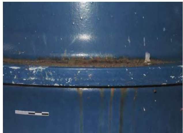
Figure 9 Detail of large blue barrel, showing corrosion at the rings. Photo: Susanne Kensche, 2013.
