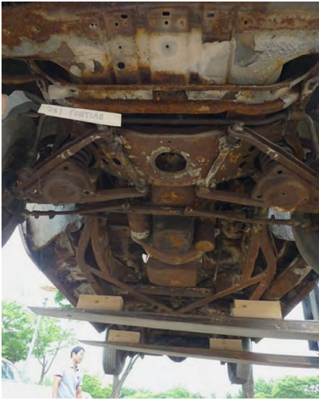
Figure 4 View of the underside of a 1955 Pontiac, showing corrosion of the car body. Photo: Zeeyoung Chin.
