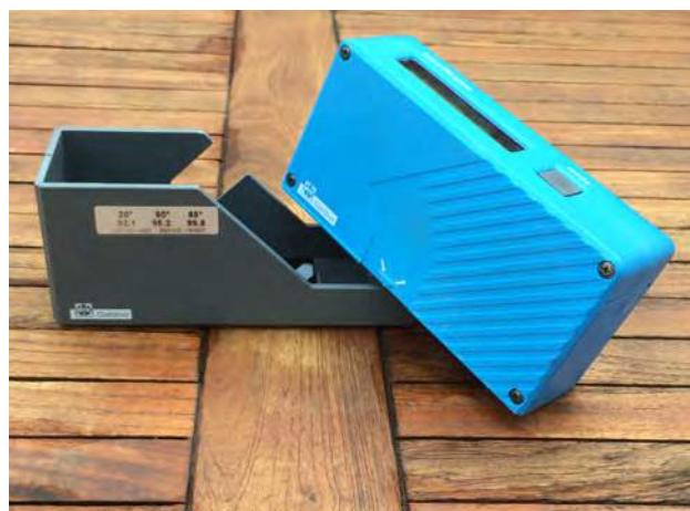
Figure 9 A glossmeter is used to measure gloss of paint, plastic, paper, and other materials. The automobile industry is a primary user of glossmeters. Photo: J. Springvloed Dubbeld.
