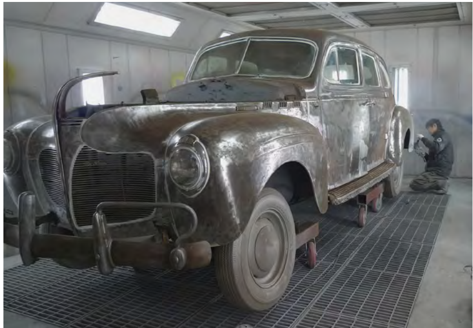
Figure 10a A 1940 DeSoto after successive layers of paint and corrosion were removed during restoration. Photo: Zeeyoung Chin.
