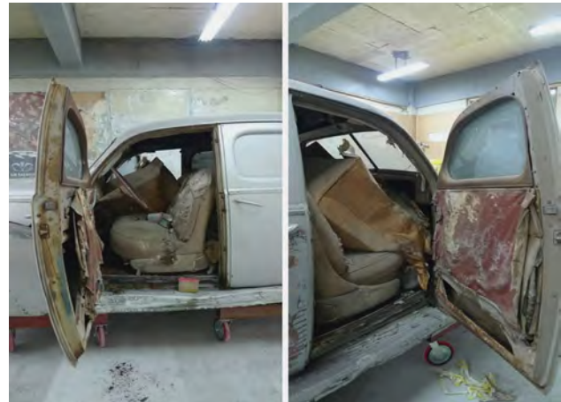
Figure 9 View of the interior of a 1937 Mercury during condition assessment. The elements were left unpacked over several years and were degrading. Left: Driver's side door. Right: Front passenger door. Photo: Zeeyoung Chin.
