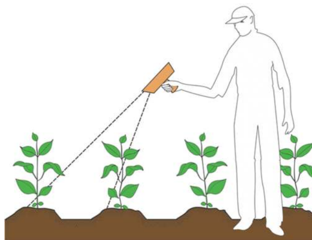
Figure 6.15. Diagram of a hand-held infrared thermometer.
