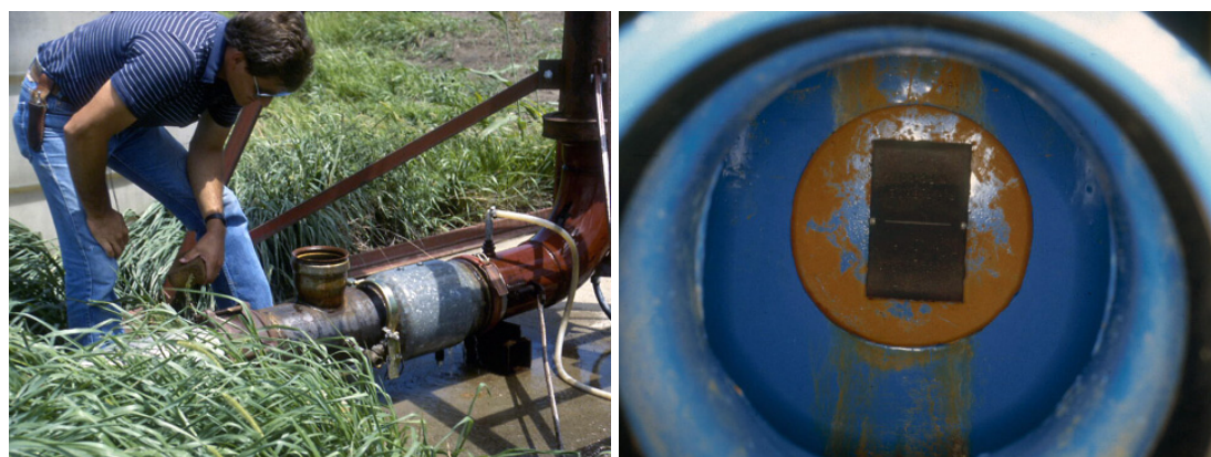
Figure 15.7. Inspection for check valve leakage in CCVA.
