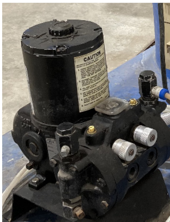
Figure 15.2. Positive displacement injection pumps: (a) piston, (b) diaphragm.
