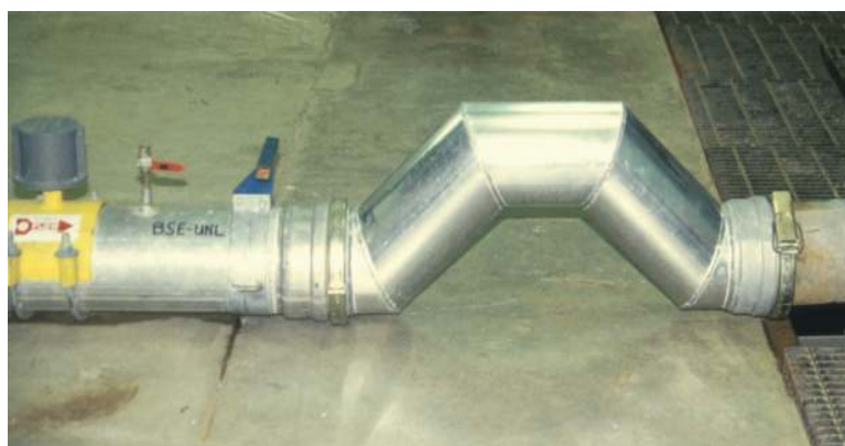
Figure 3.9. U-shaped fitting installed to guarantee full pipe flow in the meter section.
