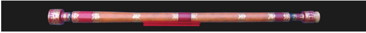
Figure 2.20 Telescope Used by Galileo. The telescope has a wooden tube covered with paper and a lens 26 millimeters across.
