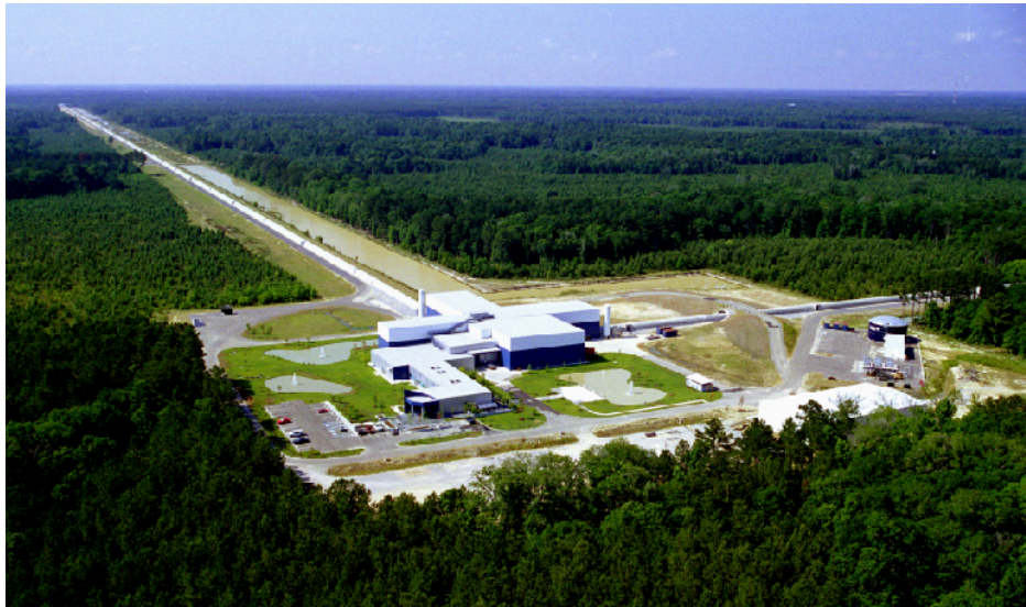
Figure 24.17 Gravitational Wave Telescope. An aerial view of the LIGO facility at Livingston, Louisiana. Extending to the upper left and far right of the image are the 4-kilometer-long detectors. (credit: modification of work by Caltech/MIT/LIGO Laboratory)
