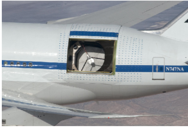
Figure 6.23 Stratospheric Observatory for Infrared Astronomy (SOFIA). SOFIA allowed observations to be made above most of Earth's atmospheric water vapor. (credit: NASA)
