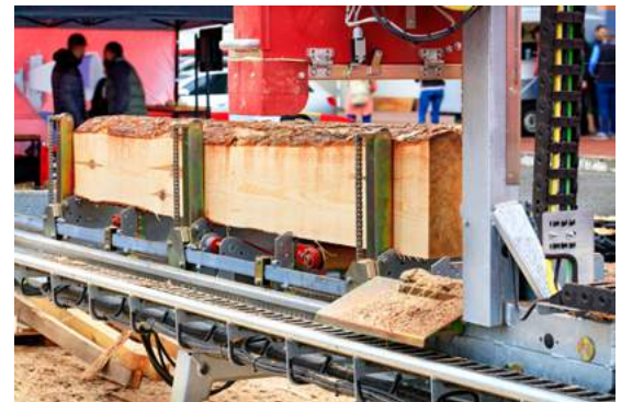
Fig.07/08 A pine log being processed on a modern automated milling machine.
