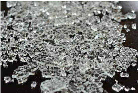
Fig.08/04 Tempered glass crumbles into small pieces instead of large shards, minimizing risk of injury.
