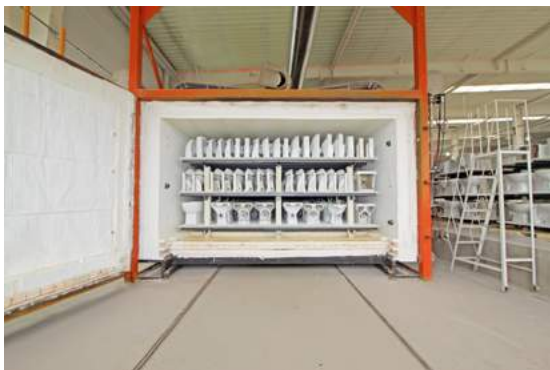
Fig.08/16 Mass-manufactured ceramic products are fired in large kilns.
