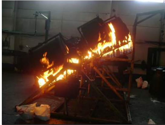
Fig.11/27 In this rotation molding example an open flame heat source is utilized.
