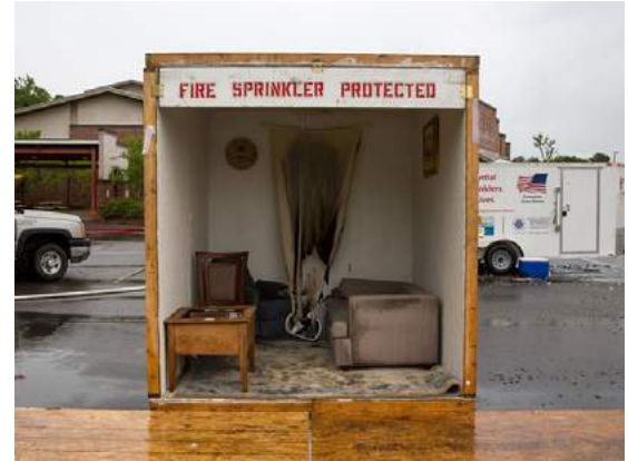
Fig.03/02 Fire sprinklers provide significant amount of protection, at a relatively reasonable cost. Especially for new construction, while lowering the fire resistance requirements for materials and assemblies.
