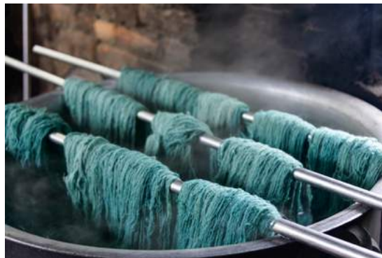
Fig.09/14 Traditional skein dyeing involves submerging the yarns in boiling dye vats.
