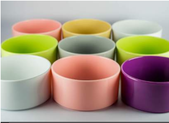
Fig.11/22 The transparency of melamine-formaldehyde resin enables a vivid representation of pigments.
