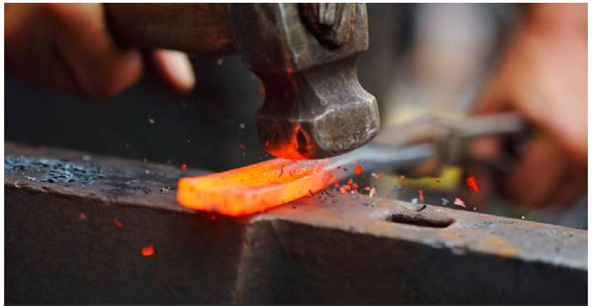
Fig.10/05 Compressing and shaping metals increases their strength and hardness while decreasing their malleability and workability.
