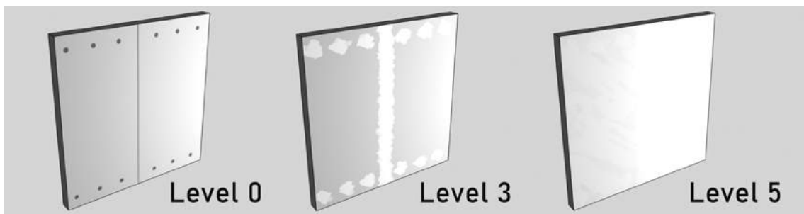
Fig.05/12 Three distinct levels of gypsum board application according to GA-214.
