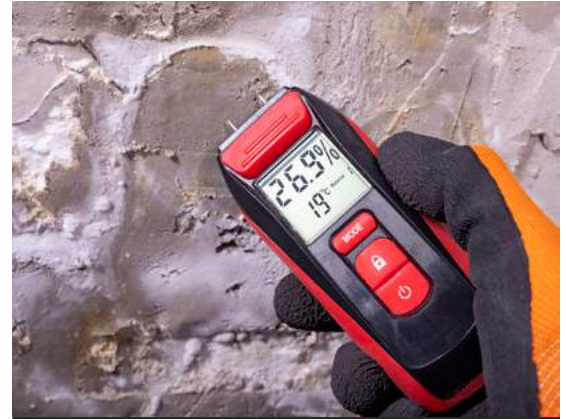
Fig.06/04 Digital hygrometers are very convenient, though the measurements can be up to 5% off.
