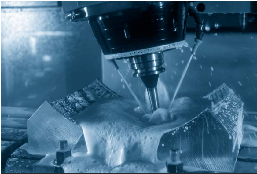
Fig.10/06 The impressive reach of a 5-axis CNC milling machine enables intricate 3d details to be fabricated.
