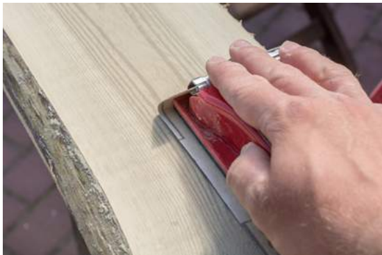
Fig.07/32 Sanding should be performed across the grain and never against the grain.
