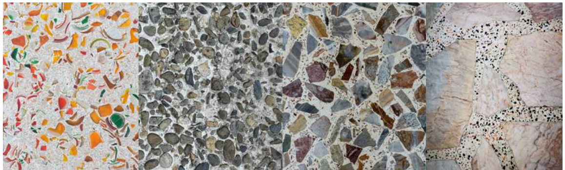
Fig.06/09 Four different terrazzo aggregates: (a) broken glass bottles, (b) unfinished pebble, (c) varying aggregate sizes, (d) large marble pieces.
