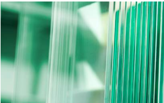
Fig.08/08 Architectural glass features a slight green tint due to iron oxide impurities.
