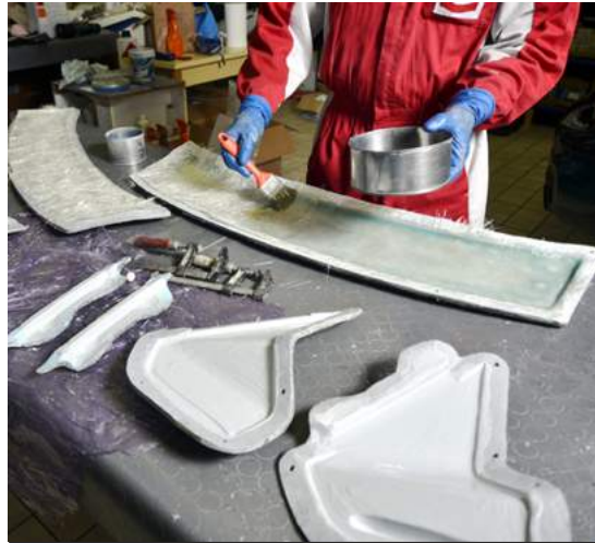
Fig.11/17 Fiberglass reinforced polyester resin is being applied to a mold.
