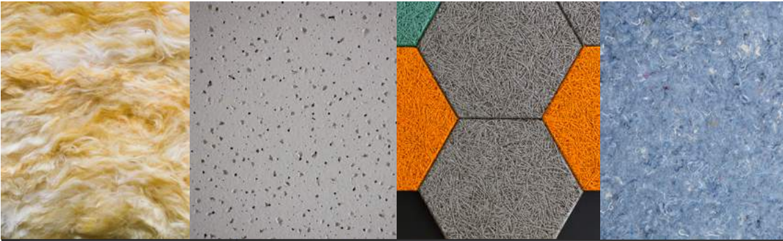
Fig.03/20 Four common sound absorptive materials: (from left to right) mineral wool, acoustic composite tile, wood wool, and recycled jean batting. Their common feature is the highly porous structure.
