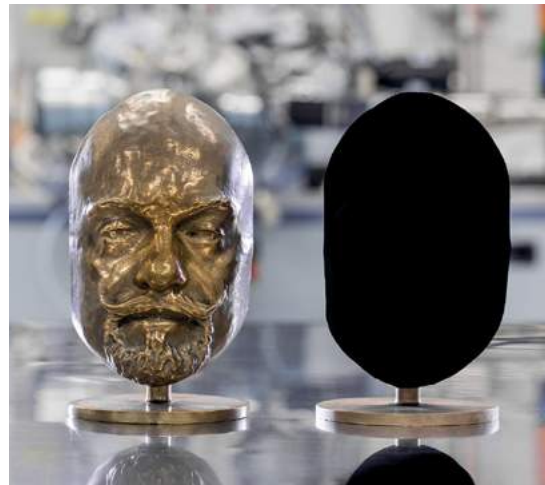
Fig.02/07 Vantablack® absorbs 99.8% of incoming light, to such an extent that surface detail can be perceived.
