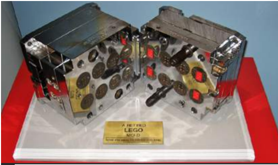
Fig.11/25 A retired Lego injection mold.
