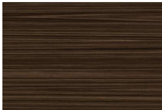
Fig.07/36 Wenge, an endangered exotic lumber, can be easily imitated with veneer reconstitution.
