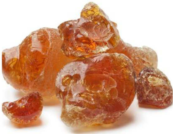
Fig.05/04 Acacia tree sap, or gum arabic, has been used as a natural paint binder for thousands of years.
