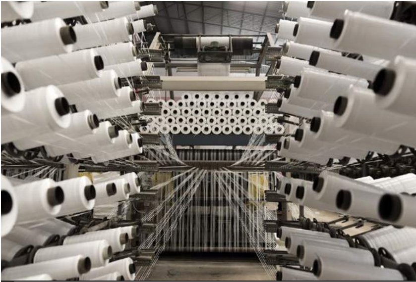
Fig.09/09 PVC fibers are being drawn and spun into spools.
