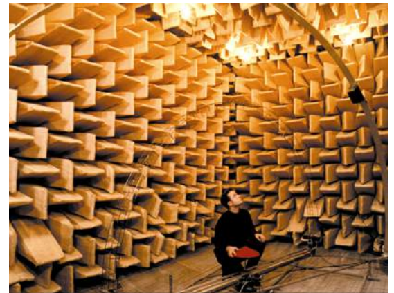
Fig.03/19 The long protrusions in an anechoic chamber are necessary for absorbing lower frequency content.
