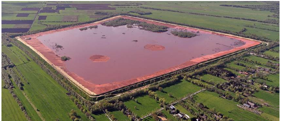
Fig.10/19 Red mud is a toxic byproduct of virgin aluminum refinement process, source of serious environmental concerns.
