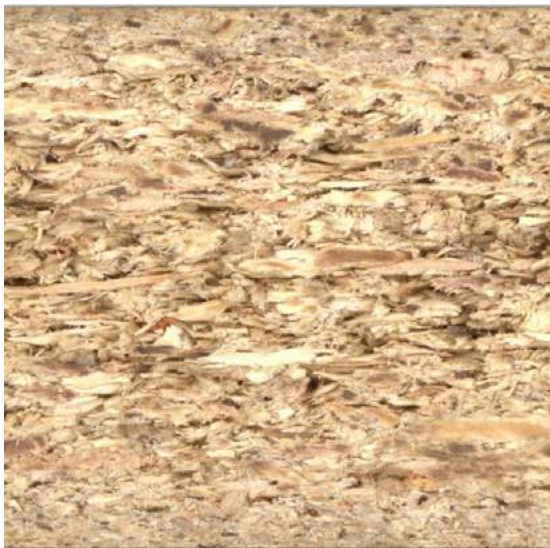
Fig.03/15 Formaldehyde is utilized as the binding resin matrix in most particleboard manufacturing.
