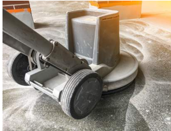
Fig.06/07 Concrete polishers, or floor grinders, feature rotating abrader pads underneath.
