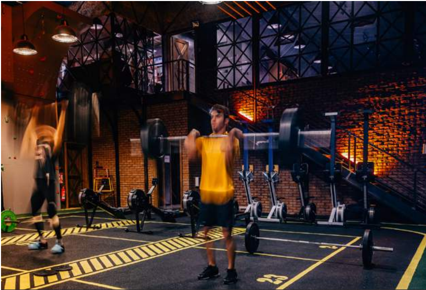
Fig.11/18 Rubber flooring is highly suitable for gym environments, where heavy loads are dropped and rolled around continuously.
