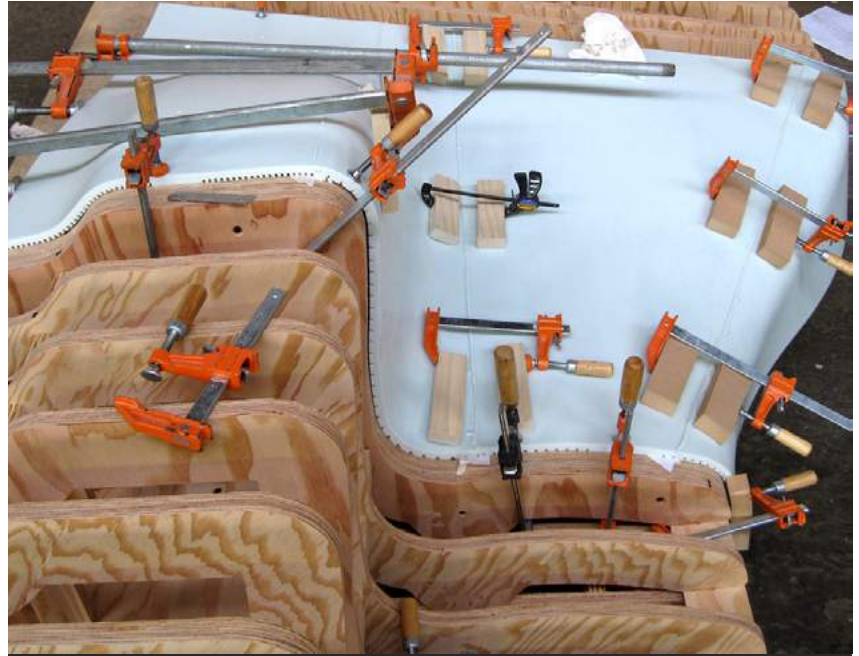
Fig.11/33 Solid surface product being bent around a plywood mold, through utilizing a mixture of heat treatment and kerfing techniques.
