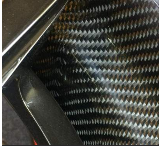
Fig.11/31 Typical carbon fiber implementation involves plain woven carbon fibers set in epoxy resin matrix.
