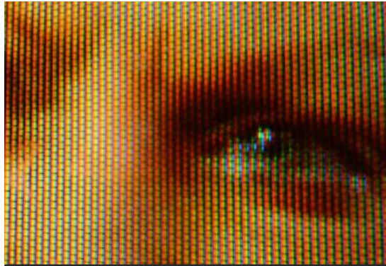
Fig.02/12 Red, green, and blue pixels light up at different intensities to form the image.
