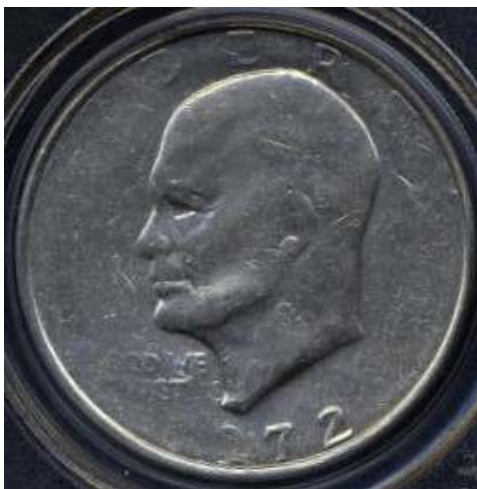
1972 Eisenhower dollar struck with partially filled-in dies. (Note: Circulated specimen but the lack of obverse details is due to a filled-in die as evidenced by the strength of the reverse design. The reverse die was also partially filled-in as evidenced by weakness on the "NE" and "D" in "ONE DOLLAR.")
