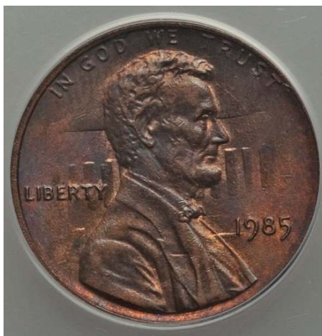
1985 Lincoln cent with clashed dies—an error nicknamed a “Prisoner Penny” as it appears Lincoln is behind bars! These raised lines surrounding Lincoln are from the spaces between the columns of the Lincoln Memorial design seen on the reverse. They were transferred to the obverse die from the reverse die when they smacked together without a planchet in between them.
