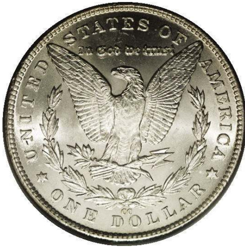
1890-CC Morgan silver dollar with a "tail bar" die gouge (right, normal reverse die left). Look under the arrow shafts for the thick line going down to the wreath, above the "E" in "ONE." A gauge on a die will show up as a raised mark on the coin struck from it.
