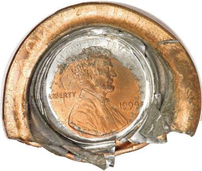
1999 Lincoln cent, three-piece bonded die cap. Three separate planchets became stuck in the coining chamber and were fused or bonded together due to the intense heat and pressure.
