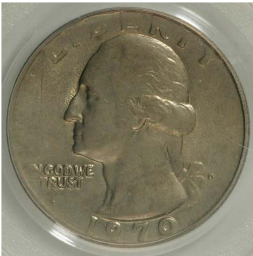
1970-D Washington quarter struck on a planchet the thickness of a dime. (Not struck on a dime planchet, but on copper-nickel stock that was rolled out for dimes. The coin was not able to receive a full/strong strike due to the thinness of the planchet. Dimes are thinner than quarters.)
