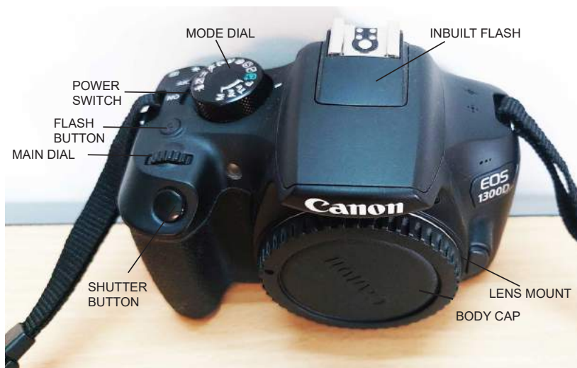
Figure 2.9: Parts of a DSLR camera (front-side)
