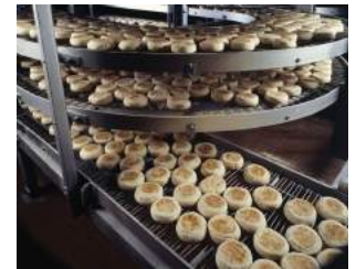
Pictured here are English muffins as they run along a conveyor belt at a bakery production plant.
