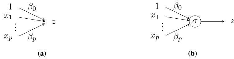
Figure 7.1: Graphical illustration of a linear regression model (Figure 7.1a), and a generalized linear regression model (Figure 7.1b). In Figure 7.1a, the output z is described as the sum of all terms \beta_0 and \{\beta_j x_j\}_{j=1}^p , as in (7.3). In Figure 7.1b, the circle denotes addition and also transformation through the activation function \sigma , as in (7.4).
