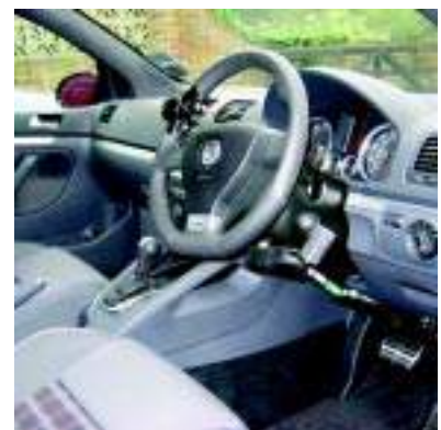
Fig 17 A example of a modified car with hand controls
