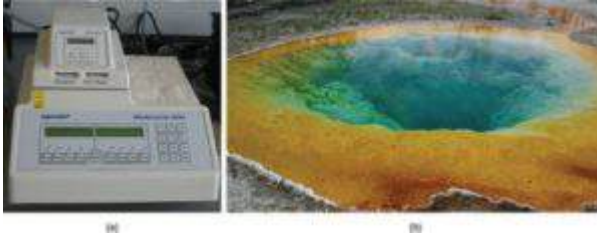
Figure 1: (a) A thermal cycler, such as the one shown here, is a basic tool used to study DNA in a process called the polymerase chain reaction (PCR). The polymerase enzyme most often used with PCR comes from a strain of bacteria that lives in (b) the hot springs of Yellowstone National Park. (credit a: modification of work by Magnus Manske; credit b: modification of work by Jon Sullivan)
