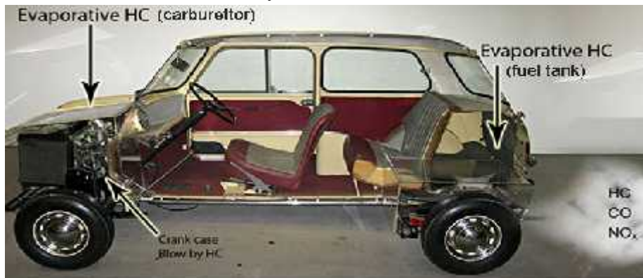
Emission sources in a gasoline fuelled car.
