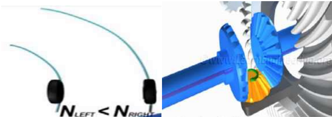
Travelling distance of wheels and direction of rotation of spider gear during left turn
