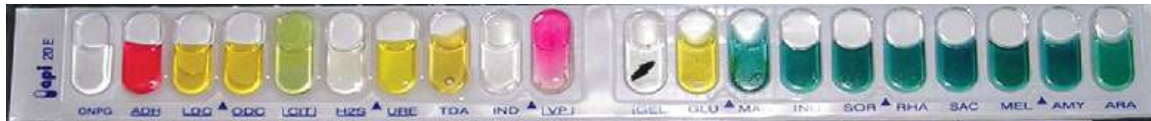
FIGURE 8.18 The API 20NE test strip is used to identify specific strains of gram-negative bacteria outside the Enterobacteriaceae. Here is an API 20NE test strip result for Photobacterium damsela ssp. piscicida .
