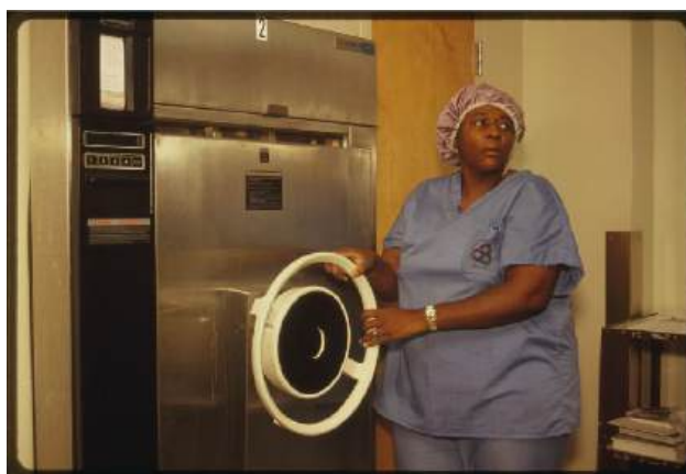
FIGURE 13.7 A technician sterilizes a sample using an autoclave. (Credit: Martha Cooper / Picryl; Public Domain.)
