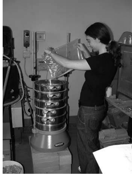
Fig 8 Laboratory test: grain size distribution (after separation of the aggregates from the binder).
