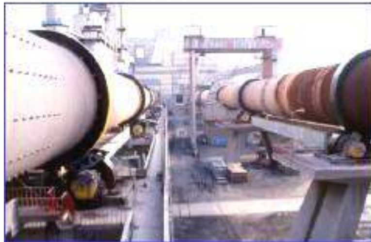
Figure 3.8: Le four cylindrique rotatif
