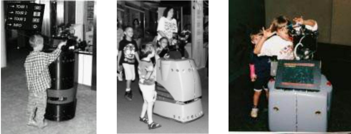
Figure 7: Probabilistic algorithms were used pervasively for the museum tour-guide robots Rhino (left image) and Minerva (right two images), which guided thousand of people through crowded museums fully autonomously.
