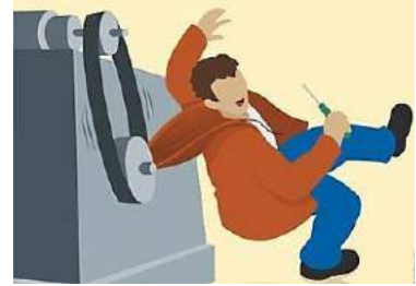
Loose Clothing Entangled Hazard
