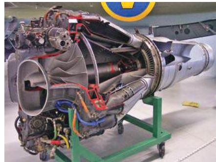
(b) De Havilland Goblin II centrifugal turbojet cut away. © Ian Dunster / Wikimedia Commons / CC-BY-SA-3.0 .
