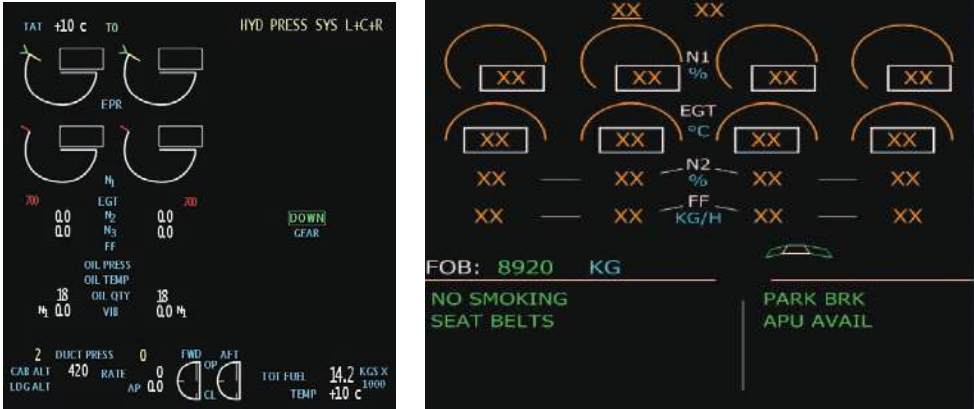
(a) EICAS display. © User:Anynobody / Wikimedia Commons / CC-BY-SA-3.0. (b) Airbus A340-300 ECAM Display. Author: User:Trainer / Wikimedia Commons / Public Domain.
