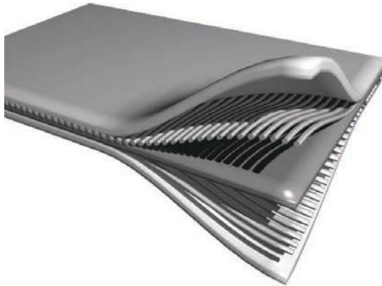
Figure 4.10: Sketch of a fibre-reinforced composite materials. © PerOX / Wikimedia Commons / Public Domain.
