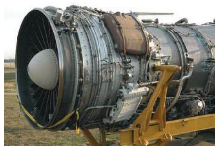
(d) Soloviev D-30KU-154 low-bypass turbofan engine. © User:VargaA / Wikimedia Commons / CC-BY-SA-3.0 .
