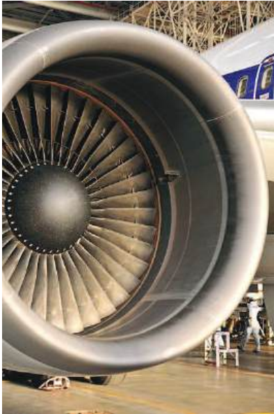
(a) The inlet of a CF6-80C2B2 turbofan engine from an All Nippon Airways aircraft in Tokyo International Airport. © Noriko SHINAGAWA / Wikimedia Commons / CC-BY-SA-2.0 .
