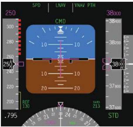
(b) Example of a typical PFD on an aircraft with glass cockpit. © User:Denelson83 / Wikimedia Commons / CC-BY-SA-3.0.
