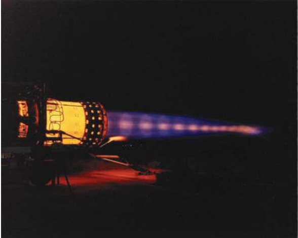
Figure 6.16: A statically mounted Pratt & Whitney J58 engine with full after-burner. Wikimedia Commons / Public Domain.
