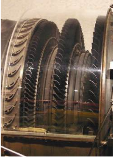
(a) The turbine rotor of a GE J79 turbojet engine. © User:Stahlkocher / Wikimedia Commons / CC-BY-SA-3.0.
