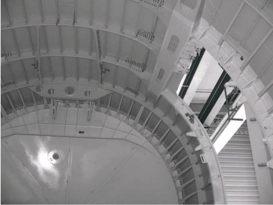
Figure 4.12: Semimonocoque Airbus A340 rear fuselage, seen from inside. © Sovxx / Wikimedia Commons / CC-BY-SA-3.0.
