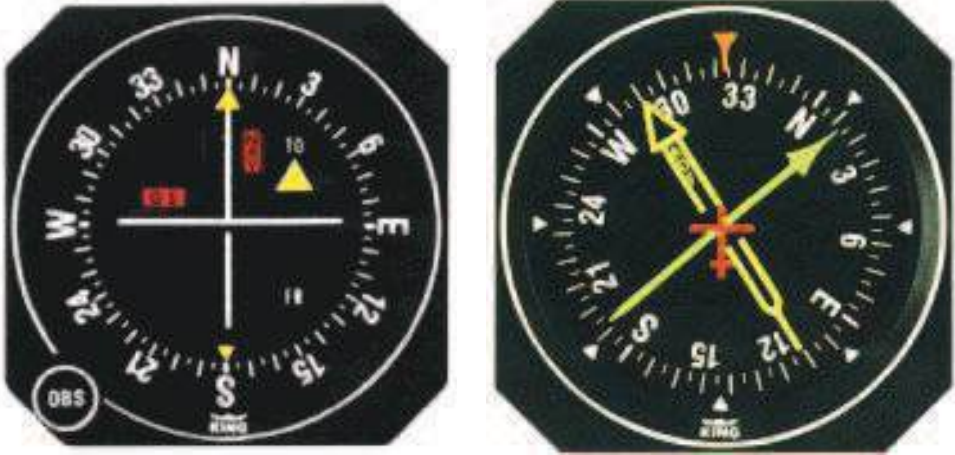
(a) An aircraft Course Deviation Indicator (CDI). (b) An aircraft Radio Magnetic Indicator (RMI). © User:Wessmann.clp / Wikimedia Commons / User:Wessmann.clp / Wikimedia Commons / GNU-3.0 . CC-BY-SA-3.0 .
