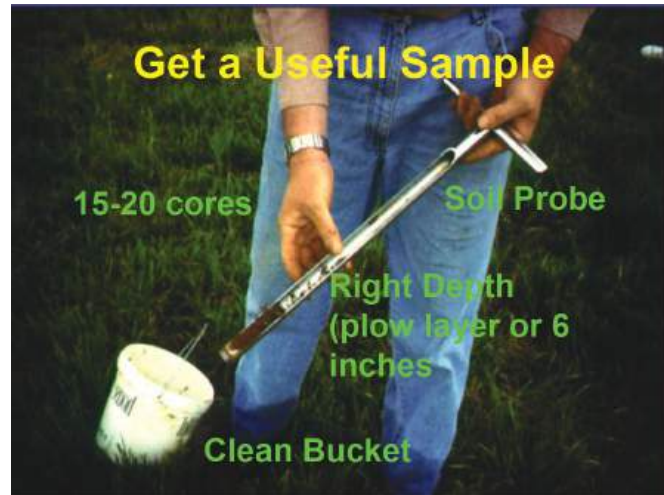
Figure 3.8. Key points of taking a good soil sample (right tool, consistent depth and enough subsamples).
