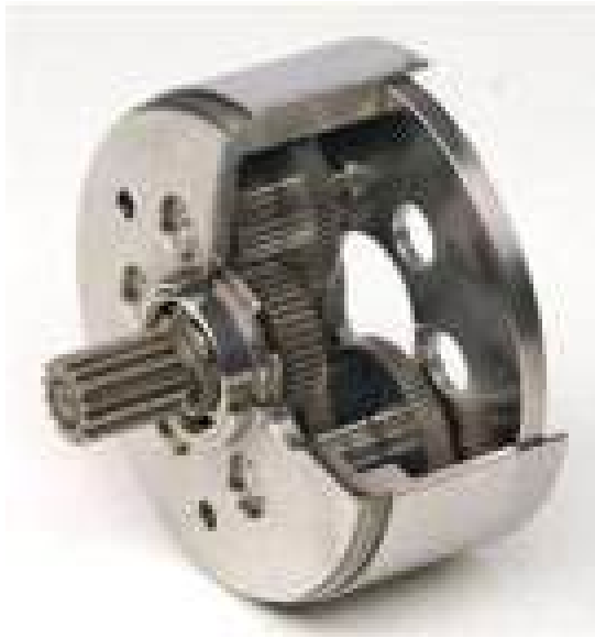
Figure 3.8 (b) Parts of overdrive
