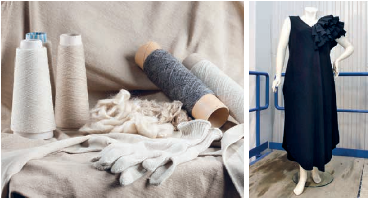
Figure 4. Carbamate fibers made from textile waste and products made from this material (photos by VTT).
