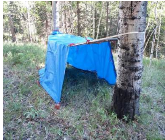
Figure 12: Lower tarp on race track loop; spreader bars create steep walls and wide floor
