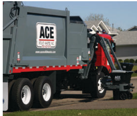
Garbage truck with automated side loader for residential waste collection, United States (ACE Solid Waste).
