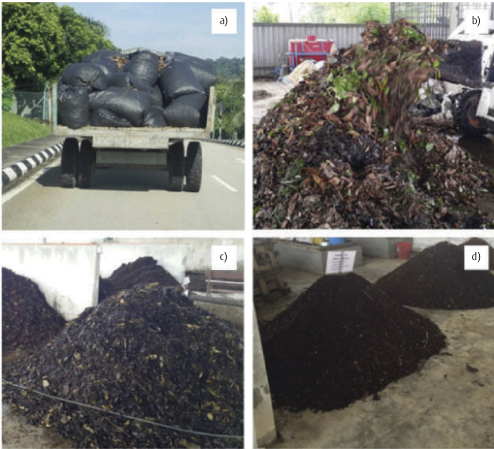
Figure 6.14 Weekly collection of yard waste in plastic bags in Serdang, Selangor, Malaysia (a); mixture of yard waste with livestock manure at the beginning of composting (b); static compost pile at 35 days (c); finished compost (d). Image: Abdul Rahman et al. (2020).
