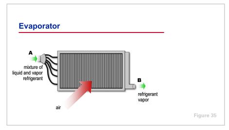
At the inlet to the **evaporator**, the refrigerant exists as a cool, low-pressure mixture of liquid and vapor. In this example, the evaporator is a finned-tube coil used to cool air. Other types of evaporators are used to cool water.
