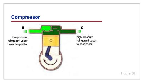
The **compressor** raises the pressure of the refrigerant vapor (**B**) to a pressure and temperature high enough (**C**) so that it can reject heat to another fluid, such as ambient air or water. There are several types of compressors. The type shown in this figure is a reciprocating compressor.
