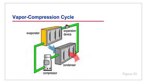
A compressor, condenser, and expansion device form the rest of the system that returns the refrigerant vapor to a low-temperature liquid, which can again be used to produce useful cooling. This cycle is called the **vapor-compression refrigeration cycle**.
