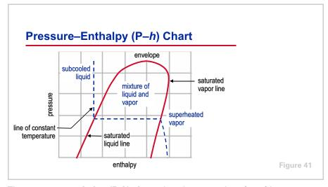
The **pressure-enthalpy** (**P-h**) **chart** plots the properties of a refrigerant—refrigerant pressure on the vertical axis and enthalpy on the horizontal axis. **Enthalpy** is a measure of heat quantity, both sensible and latent, per pound [kg] of refrigerant. It is typically expressed in terms of Btu/lb [kJ/kg].
