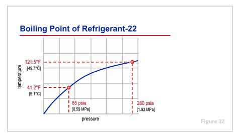
This curve illustrates the pressures and corresponding temperatures at which R-22 boils and condenses. At a pressure of 85 psia [0.59 MPa], the liquid R-22 will boil at 41.2°F [5.1°C]. As an example, assume that a compressor is used to
