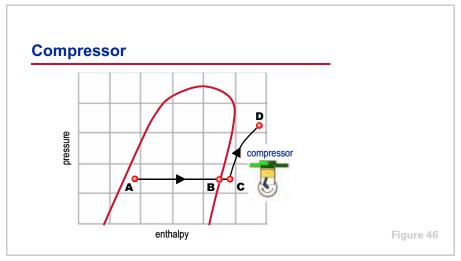
The compressor draws in the superheated refrigerant vapor (**C**) and compresses it to a pressure and temperature (**D**) high enough that it can reject heat to another fluid. As the volume of the refrigerant is reduced by the compressor, its pressure is increased. Additionally, the mechanical energy used by the compressor to accomplish this task is converted to heat energy. This causes the temperature of the refrigerant to also rise as its pressure is increased.
