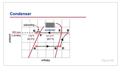
Inside of the condenser, heat is transferred from the hot, high-pressure refrigerant vapor (**D**) to relatively cool ambient air. This reduction in the enthalpy of the refrigerant vapor causes it to desuperheat. It becomes saturated vapor, condenses into saturated liquid, and further subcools before leaving the condenser (**G**) to go to the expansion device.
