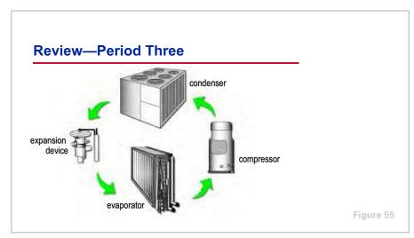
Period Three presented the basic vapor-compression refrigeration cycle, and specifically the use of a compressor, condenser, and expansion device to "recover" the evaporated refrigerant and complete the cycle. The primary components of the vapor-compression refrigeration cycle include the evaporator, compressor, condenser, and expansion device.
