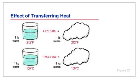
In fact, 970.3 Btu must be added to 1 lb of 212°F water to completely transform it to 1 lb of steam at the same temperature.
