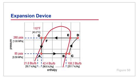
The temperature of the refrigerant entering the expansion device (**G**) is 110°F [43.3°C] and its pressure is 280 psia [1.93 MPa]. (The refrigerant condensed at 121.5°F [49.7°C] and was subcooled to 110°F [43.3°C].) The enthalpy of the refrigerant at this condition is 42.4 Btu/lb [98.6 kJ/kg]. As mentioned previously, there is no change in enthalpy during the expansion process—it is the same at both **G** and **A**.
