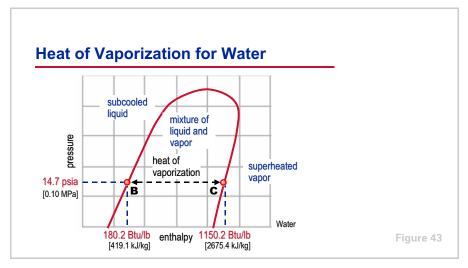
The distance between the edges of the envelope indicates the quantity of heat required to transform saturated liquid into saturated vapor at a given pressure. This is called the **heat of vaporization**.
