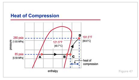
When the refrigerant vapor is discharged from the compressor, its temperature is substantially higher than its saturation temperature (the temperature at which the refrigerant would condense). The increase in enthalpy from **C** to **D** is due to heat added by the compressor, or the **heat of compression**.
