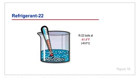
Finally, Refrigerant-22 (R-22) is a chemical used in many refrigeration systems. If, hypothetically, an open container of liquid R-22 were placed in the frozen display case, when exposed to atmospheric pressure, it would absorb heat and boil violently at -41.4°F [-40.8°C].
