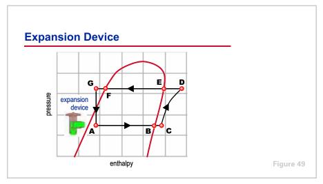
The primary purpose of the expansion device is to drop the pressure of the liquid refrigerant to equal the evaporator pressure. At this lower pressure, the refrigerant is now inside the saturation envelope where it exists as a mixture of liquid and vapor.
