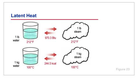
The quantity of heat that must be added to the water in order for it to evaporate cannot be sensed by an ordinary thermometer. This is because both the water and steam remain at the same temperature during this phase change.
