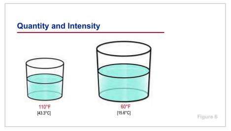
These two different masses of water contain the same quantity of heat, yet the temperature of the water on the left is higher. Why? The water on the left contains more heat per unit of mass than the water on the right. In other words, the heat energy within the water on the left is more concentrated, or intense, resulting in the higher temperature. Note that the temperature of a substance does not reveal the quantity of heat that it contains.
