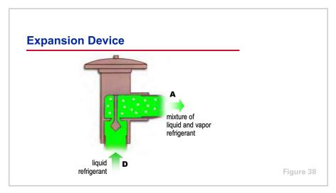
The primary purpose of the **expansion device** is to drop the pressure of the liquid refrigerant to equal the pressure in the evaporator. Several types of expansion devices can be used. The device shown is an expansion valve.
