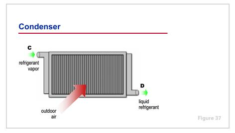
The **condenser** is a heat exchanger used to reject the heat of the refrigerant to another medium. The example shown is an air-cooled condenser that rejects heat to the ambient air. Other types of condensers are used to reject heat to water.
