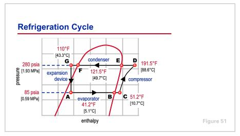
This cool mixture of liquid and vapor refrigerant leaving the expansion device then enters the evaporator (A) to repeat the cycle.
