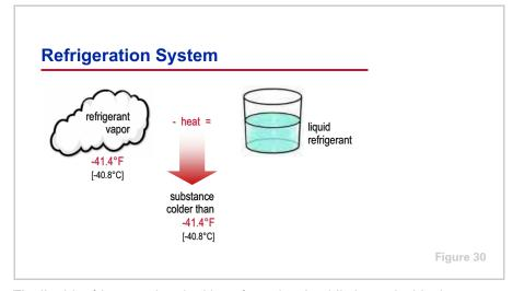
The liquid refrigerant absorbed heat from the air while it was inside the evaporator, and was transformed into a vapor in the process of doing useful cooling. Earlier in this clinic, we demonstrated that if the heat is then removed from this vapor, it will transform (condense) back to its original liquid phase.
