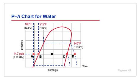
To further demonstrate the use of the P-h chart, let us look at the process of heating and boiling water, at a constant pressure, on a P-h chart for water.
