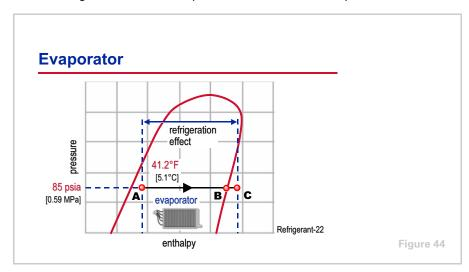
The P-h chart can be used to analyze the vapor-compression refrigeration cycle and determine the conditions of the refrigerant at any point in the cycle. The chart in this example is for R-22.
