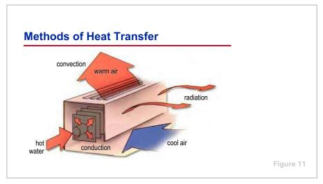
The third principle is that heat is transferred from one substance to another by one of three basic processes: conduction, convection, and radiation. The device shown is a baseboard convector that is commonly used for heating a space. It can be used to demonstrate all three processes of transferring heat.
