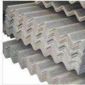
Asbestos Cement sheets
