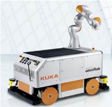
Figura 10. KMR = Mobile platform + LBR iiwa
