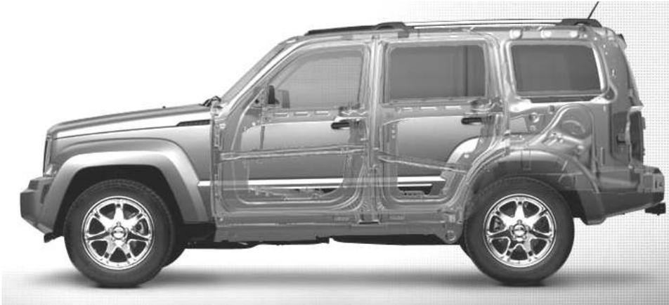
Caja de seguridad. Fuente: [www.jeep.com/.../occupant\\_protection/](http://www.jeep.com/.../occupant_protection/)
