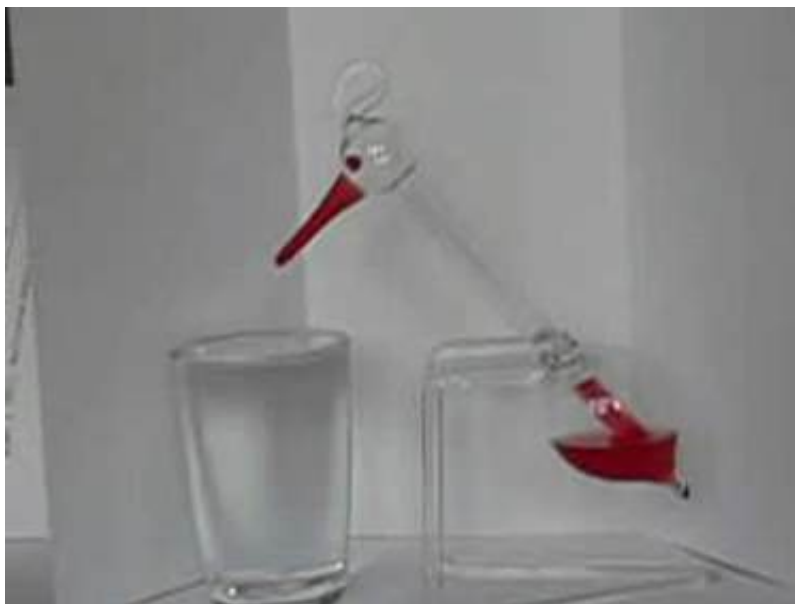
FIGURE 15.20 This novelty toy, known as the drinking bird, is an example of Carnot's engine. It contains methylene chloride (mixed with a dye) in the abdomen, which boils at a very low temperature—about 100°F. To operate, one gets the bird's head wet. As the water evaporates, fluid moves up into the head, causing the bird to become top-heavy and dip forward back into the water. This cools down the methylene chloride in the head, and it moves back into the abdomen, causing the bird to become bottom heavy and tip up. Except for a very small input of energy—the original head-wetting—the bird becomes a perpetual motion machine of sorts. (credit: Arabesk.nl, Wikimedia Commons)
