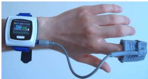
FIGURE 7.24 A pulse oximeter is an apparatus that measures the amount of oxygen in blood. A knowledge of oxygen and carbon dioxide levels indicates a person's metabolic rate, which is the rate at which food energy is converted to another form. Such measurements can indicate the level of athletic conditioning as well as certain medical problems. (credit: UusiAjaja, Wikimedia Commons)
