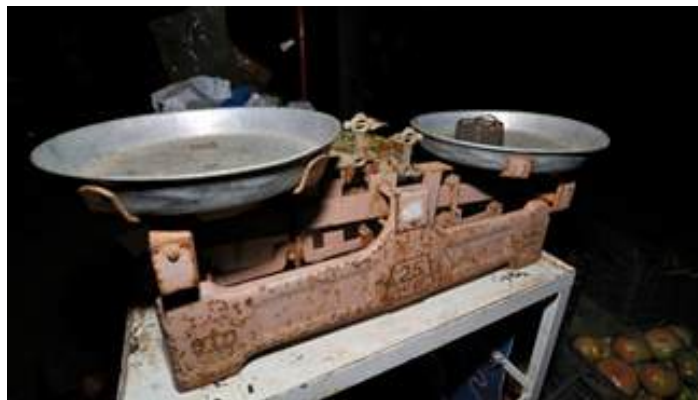
FIGURE 1.21 A double-pan mechanical balance is used to compare different masses. Usually an object with unknown mass is placed in one pan and objects of known mass are placed in the other pan. When the bar that connects the two pans is horizontal, then the masses in both pans are equal. The “known masses” are typically metal cylinders of standard mass such as 1 gram, 10 grams, and 100 grams. (credit: Serge Melki)
