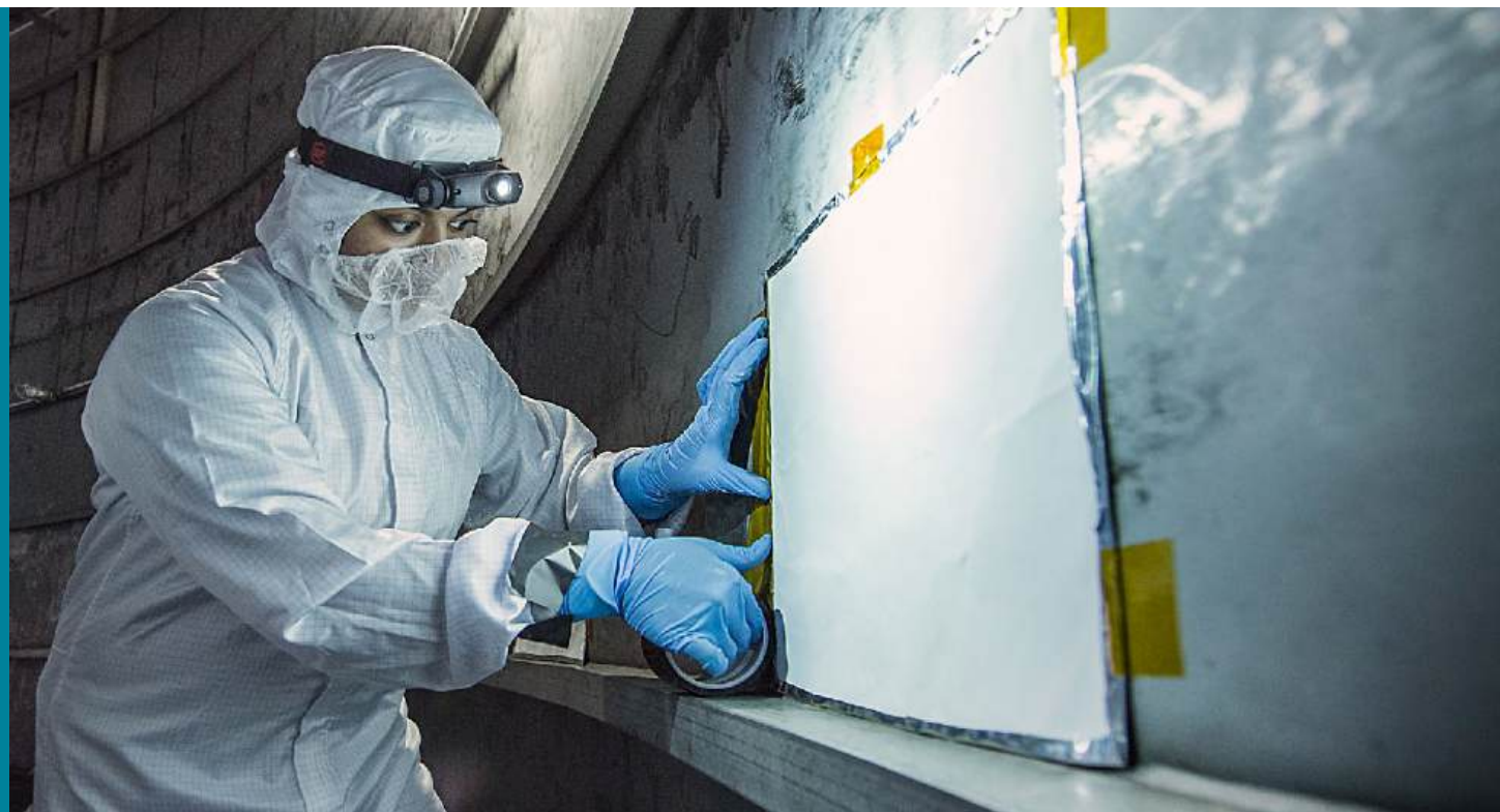
FIGURE 13.1 Molecules dissolved in surfaces undergo a process of outgassing, or release into the space around them. In a car, this leads to the famous "new car smell." In precision instruments like telescopes, this leads to major distortions due to contamination. NASA engineer Nithin Abraham created a coating to absorb these contaminants. Here she is pictured securing a coated panel beneath the Johnson Space Center's Chamber A, where it was used during testing of the James Webb Space Telescope. (credit: NASA, Chris Gunn/Flickr)
