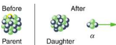
FIGURE 31.15 Alpha decay is the separation of a {}^4\text{He} nucleus from the parent. The daughter nucleus has two fewer protons and two fewer neutrons than the parent. Alpha decay occurs spontaneously only if the daughter and {}^4\text{He} nucleus have less total mass than the parent.
