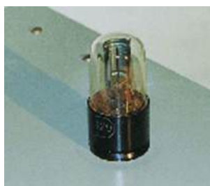
FIGURE 29.6 The photoelectric effect can be observed by allowing light to fall on the metal plate in this evacuated tube. Electrons ejected by the light are collected on the collector wire and measured as a current. A retarding voltage between the collector wire and plate can then be adjusted so as to determine the energy of the ejected electrons. For example, if it is sufficiently negative, no electrons will reach the wire. (credit: P.P. Urone)
