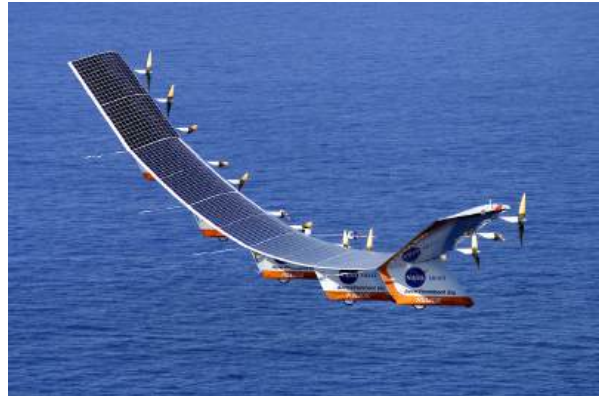
FIGURE 7.19 Solar energy is converted into electrical energy by solar cells, which is used to run a motor in this solar-power aircraft. (credit: NASA)
