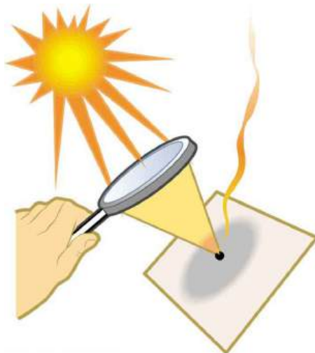
FIGURE 25.26 Sunlight focused by a converging magnifying glass can burn paper. Light rays from the sun are nearly parallel and cross at the focal point of the lens. The more powerful the lens, the closer to the lens the rays will cross.
