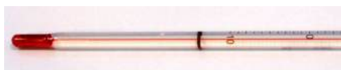
FIGURE 13.2 In a typical thermometer like this one, the alcohol, with a red dye, expands more rapidly than the glass containing it. When the thermometer's temperature increases, the liquid from the bulb is forced into the narrow tube, producing a large change in the length of the column for a small change in temperature. (credit: Chemical Engineer, Wikimedia Commons)
