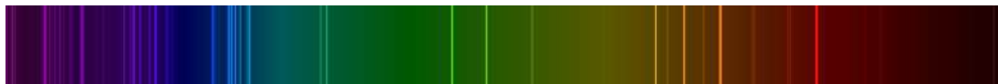
FIGURE 29.5 Emission spectrum of oxygen. When an electrical discharge is passed through a substance, its atoms and molecules absorb energy, which is reemitted as EM radiation. The discrete nature of these emissions implies that the energy states of the atoms and molecules are quantized. Such atomic spectra were used as analytical tools for many decades before it was understood why they are quantized. (credit: Teravolt, Wikimedia Commons)
