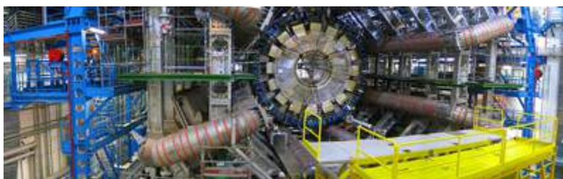
FIGURE 4.26 The world's largest particle accelerator spans the border between Switzerland and France. Two beams, traveling in opposite directions close to the speed of light, collide in a tube similar to the central tube shown here. External magnets determine the beam's path. Special detectors will analyze particles created in these collisions. Questions as broad as what is the origin of mass and what was matter like the first few seconds of our universe will be explored. This accelerator began preliminary operation in 2008. (credit: Frank Hommes)
