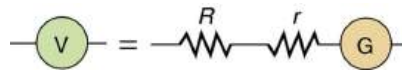
FIGURE 21.29 A large resistance R placed in series with a galvanometer G produces a voltmeter, the full-scale deflection of which depends on the choice of R . The larger the voltage to be measured, the larger R must be. (Note that r represents the internal resistance of the galvanometer.)
