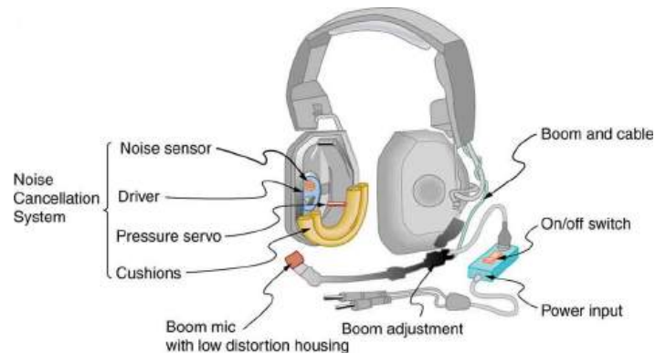
FIGURE 17.21 Headphones designed to cancel noise with destructive interference create a sound wave exactly opposite to the incoming sound. These headphones can be more effective than the simple passive attenuation used in most ear protection. Such headphones were used on the record-setting, around the world nonstop flight of the Voyager aircraft to protect the pilots' hearing from engine noise.
