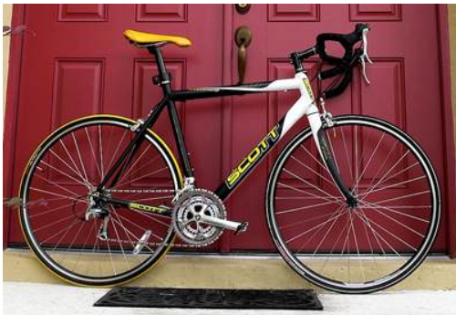
FIGURE 10.30 The image shows a side view of a racing bicycle. Can you see evidence in the design of the wheels on this racing bicycle that their moment of inertia has been purposely reduced? (credit: Jesús Rodríguez)
