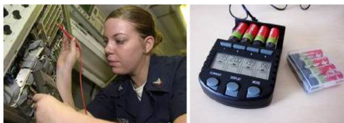
FIGURE 21.13 These two battery testers measure terminal voltage under a load to determine the condition of a battery. The large device is being used by a U.S. Navy electronics technician to test large batteries aboard the aircraft carrier USS Nimitz and has a small resistance that can dissipate large amounts of power. (credit: U.S. Navy photo by Photographer's Mate Airman Jason A. Johnston) The small device is used on small batteries and has a digital display to indicate the acceptability of their terminal voltage. (credit: Keith Williamson)
