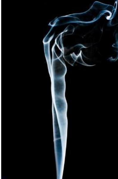
FIGURE 12.10 Smoke rises smoothly for a while and then begins to form swirls and eddies. The smooth flow is called laminar flow, whereas the swirls and eddies typify turbulent flow. If you watch the smoke (being careful not to breathe on it), you will notice that it rises more rapidly when flowing smoothly than after it becomes turbulent, implying that turbulence poses more resistance to flow. (credit: Creativity103)
