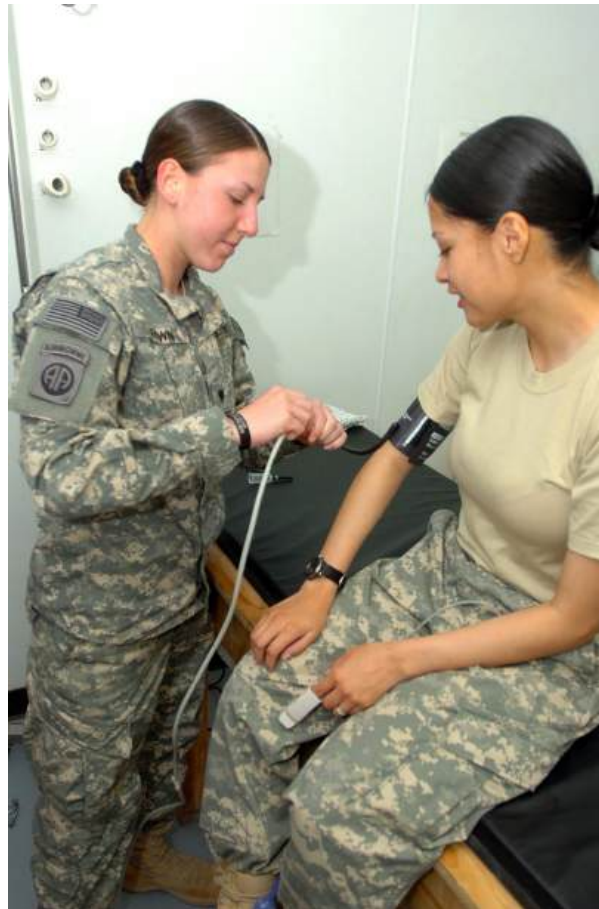
FIGURE 11.15 In routine blood pressure measurements, an inflatable cuff is placed on the upper arm at the same level as the heart. Blood flow is detected just below the cuff, and corresponding pressures are transmitted to a mercury-filled manometer. (credit: U.S. Army photo by Spc. Micah E. Clare\4TH BCT)
