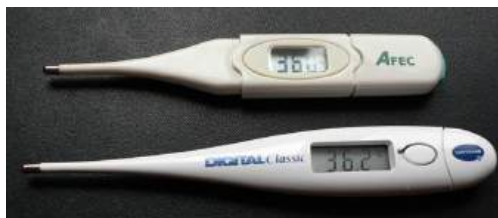
FIGURE 20.12 These familiar thermometers are based on the automated measurement of a thermistor's temperature-dependent resistance. (credit: Biol, Wikimedia Commons)
