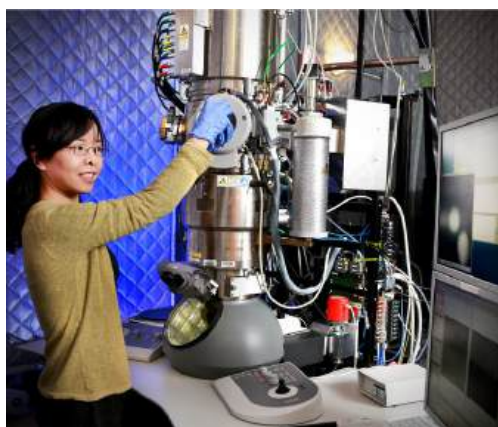
FIGURE 26.21 An electron microscope has the capability to image individual atoms on a material. The microscope uses vacuum technology, sophisticated detectors and state of the art image processing software. Researchers use the devices in their work on biological and, in the case of Miaofang Chi (pictured), lithium ion battery materials and fuel cell catalysts. (credit: Oak Ridge National Laboratory)
