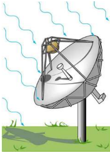
FIGURE 24.27 Satellite dishes receive TV signals sent from orbit. Although the signals are quite weak, the receiver can detect them by being tuned to resonate at their frequency.
