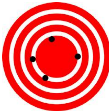
FIGURE 1.23 A GPS system attempts to locate a restaurant at the center of the bull's-eye. The black dots represent each attempt to pinpoint the location of the restaurant. The dots are spread out quite far apart from one another, indicating low precision, but they are each rather close to the actual location of the restaurant, indicating high accuracy. (credit: Dark Evil)
