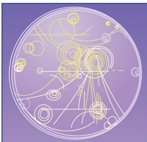
FIGURE 22.18 Trails of bubbles are produced by high-energy charged particles moving through the superheated liquid hydrogen in this artist's rendition of a bubble chamber. There is a strong magnetic field perpendicular to the page that causes the curved paths of the particles. The radius of the path can be used to find the mass, charge, and energy of the particle.
