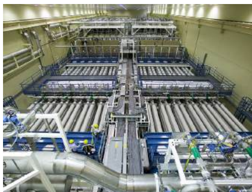
FIGURE 32.19 National Ignition Facility (CA). This image shows a laser bay where 192 laser beams will focus onto a small D-T target, producing fusion. (credit: Lawrence Livermore National Laboratory, Lawrence Livermore National Security, LLC, and the Department of Energy)
