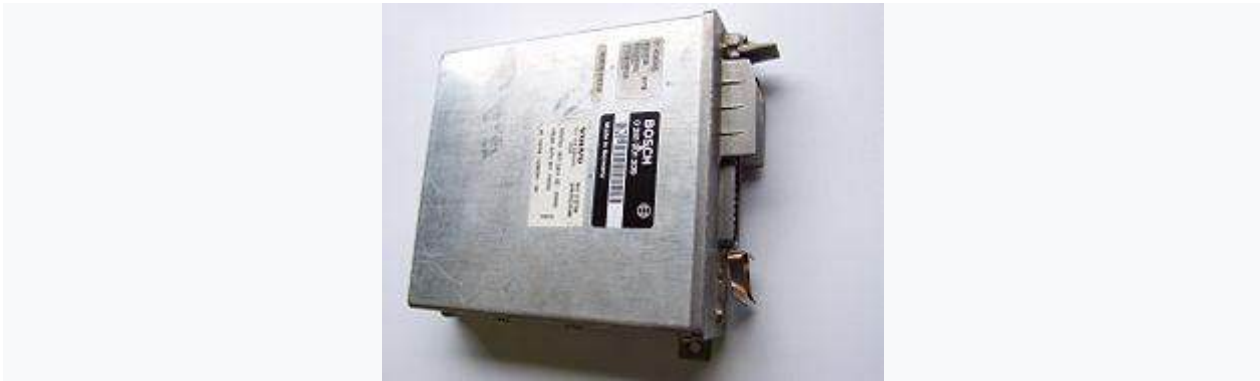
Edc control unit
