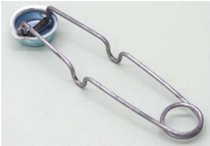
78: Cutting Torch Sparkers: These little spring-loaded sparkers (which have replaceable flints) are used for lighting gas torches, but they will also light most tinders as well as any other spark-based technique.
