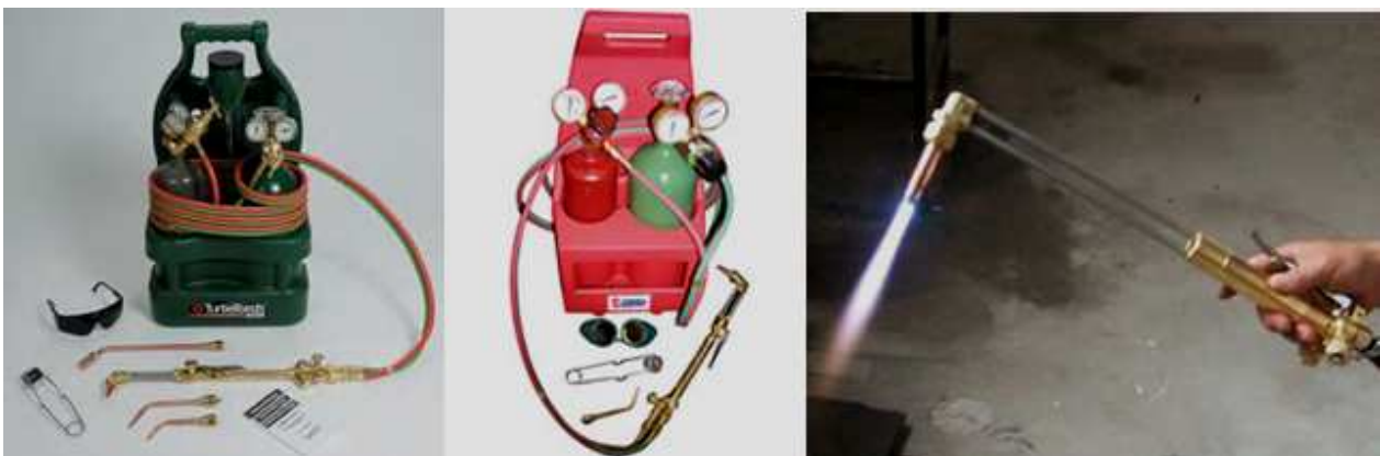
77: Cutting and Welding Torches: Oxy-acetylene torches use a combination of acetylene gas and oxygen, to produce a flame that will cut through steel plate (and set things on fire). The gas is usually lit by a separate sparker tool (see # 78), but any other ignition source will also work.
