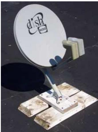
19: Improvised parabolic reflector (satellite dish and foil): Any satellite dish can be used as a larger parabolic reflector, by covering the inner curved surface with foil, and then aiming it towards the sun. But be careful when finding the focal spot, as larger reflectors can create enough heat to be dangerous.
