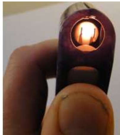
79: Electric Cigarette Lighters: Nowadays you can buy tiny battery-powered electric cigarette lighters, which use small heating elements to set cigarettes on fire. They will also ignite any good tinder.
