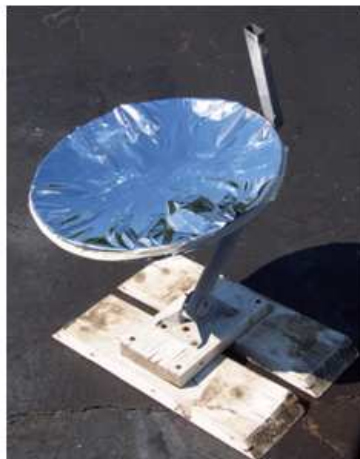
19: Improvised parabolic reflector (satellite dish and foil): Any satellite dish can be used as a larger parabolic reflector, by covering the inner curved surface with foil, and then aiming it towards the sun. But be careful when finding the focal spot, as larger reflectors can create enough heat to be dangerous.
