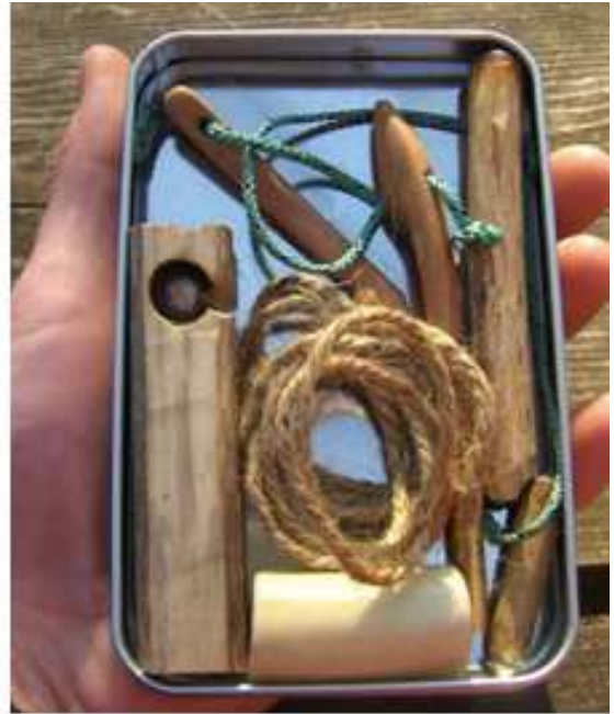
44: Fire Bow Drill (collapsible): Since the bow of a bow drill doesn't flex like an archery bow (it just holds both ends of the cord), you can make a collapsible bow that can be stored in a small space. Like a collapsible spindle stick for a hand drill, the collapsible bow can have a socket made from bamboo, or metal tubing.
