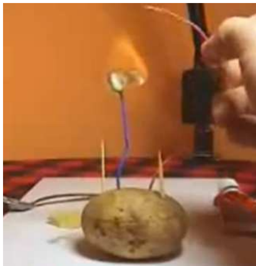
82: Electricity and Battery Power (improvised batteries, & flammable-soaked tinder): If you know enough basic chemistry to make an improvised battery, you can use the spark to ignite some tinder. Weak batteries make weak sparks, so for best results coat your tinder with some flammable fuel.
