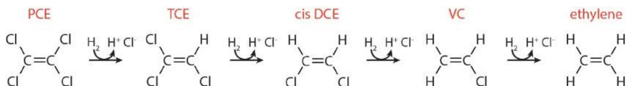
Figure 14.10 Sequential removal of chlorine during organohalide respiration with dihydrogen as the electron donor. Acronyms are defined in Table 14.1. At each step, two electrons from dihydrogen oxidation are added to the organohalide, reducing it and causing its chlorine atoms to be replaced by hydrogens. https://commons.wikimedia.org/wiki/File:Organohalide_respiration.jpg
