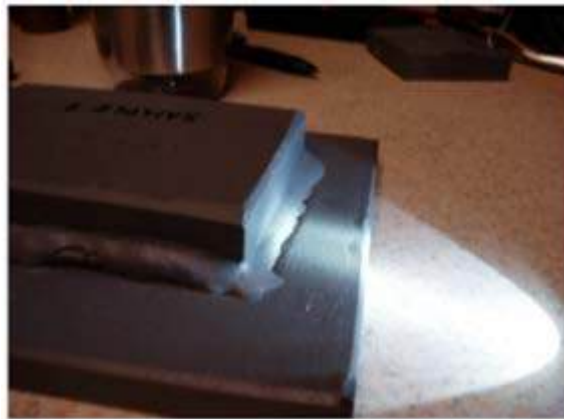
Figure 33: Visual inspection with flashlight
