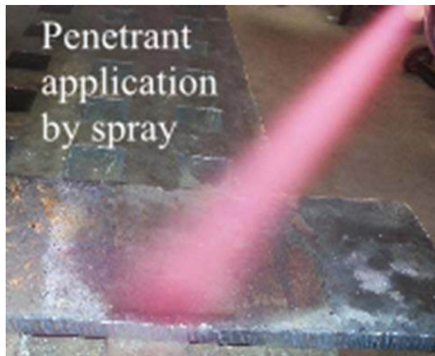
Figure 17: Application of penetrant
