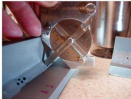
Figure 16: Throat measurement with cam gauge
