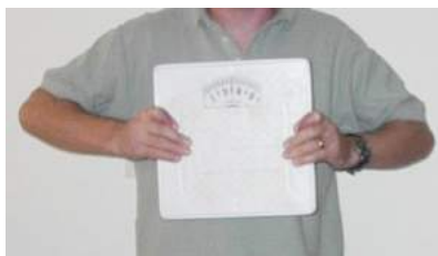
l / I squeeze the bathroom scale. It does make sense to add my fingers' force to my thumbs', because they both act on the same object — the scale.
