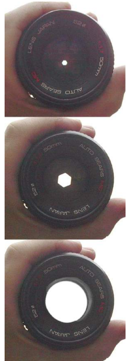
d/The same lens is shown with its diaphragm set to three different apertures.
