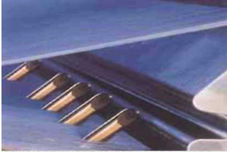
Figure 21. Relay nozzles on an air jet weaving machine
