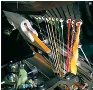
Figure 18. Rigid rapier machine with selection of 12 weft yarns (courtesy of Dornier)
