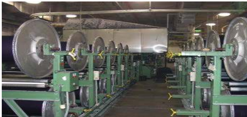
Figure 5. Slasher creel loaded with 12 section beams for weaving denim
