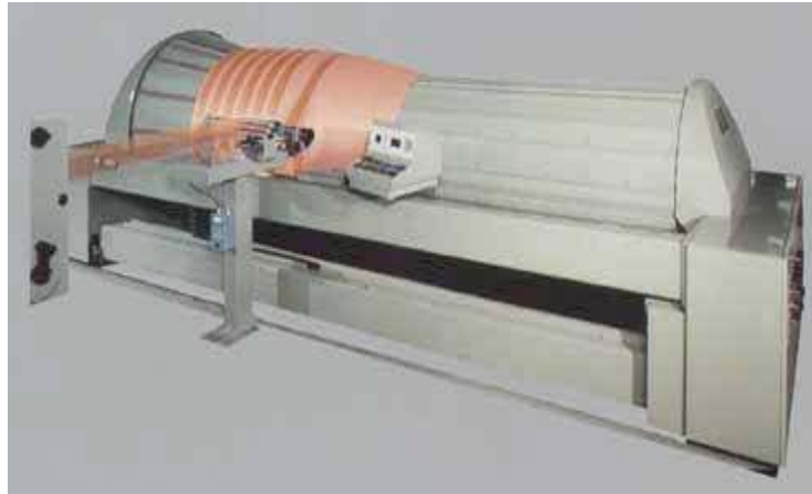
Figure 3. Indirect warping of bands or sections of yarn onto a pattern drum
