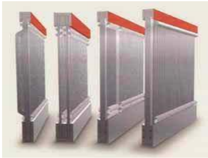
Figure 23. Various reeds for different fabric constructions
