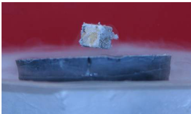
Figure 9.28 A small, strong magnet levitates over a superconductor cooled to liquid nitrogen temperature. The magnet levitates because the superconductor excludes magnetic fields. (credit: Joseph J. Trout)
