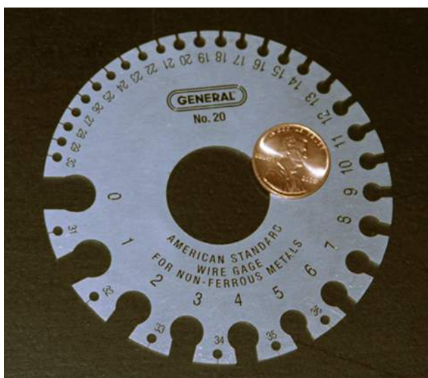
Figure 9.11 A device for measuring the gauge of electrical wire. As you can see, higher gauge numbers indicate thinner wires. (credit: Joseph J. Trout)
