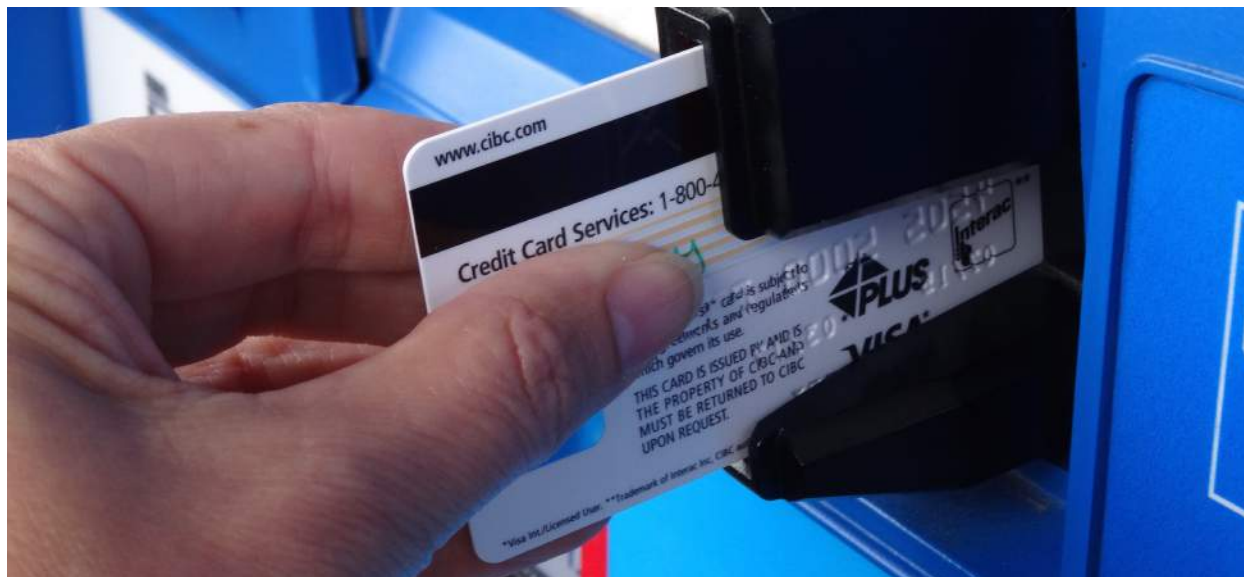
Figure 13.1 The black strip found on the back of credit cards and driver's licenses is a very thin layer of magnetic material with information stored on it. Reading and writing the information on the credit card is done with a swiping motion. The physical reason why this is necessary is called electromagnetic induction and is discussed in this chapter. (credit: modification of work by Jane Whitney)
