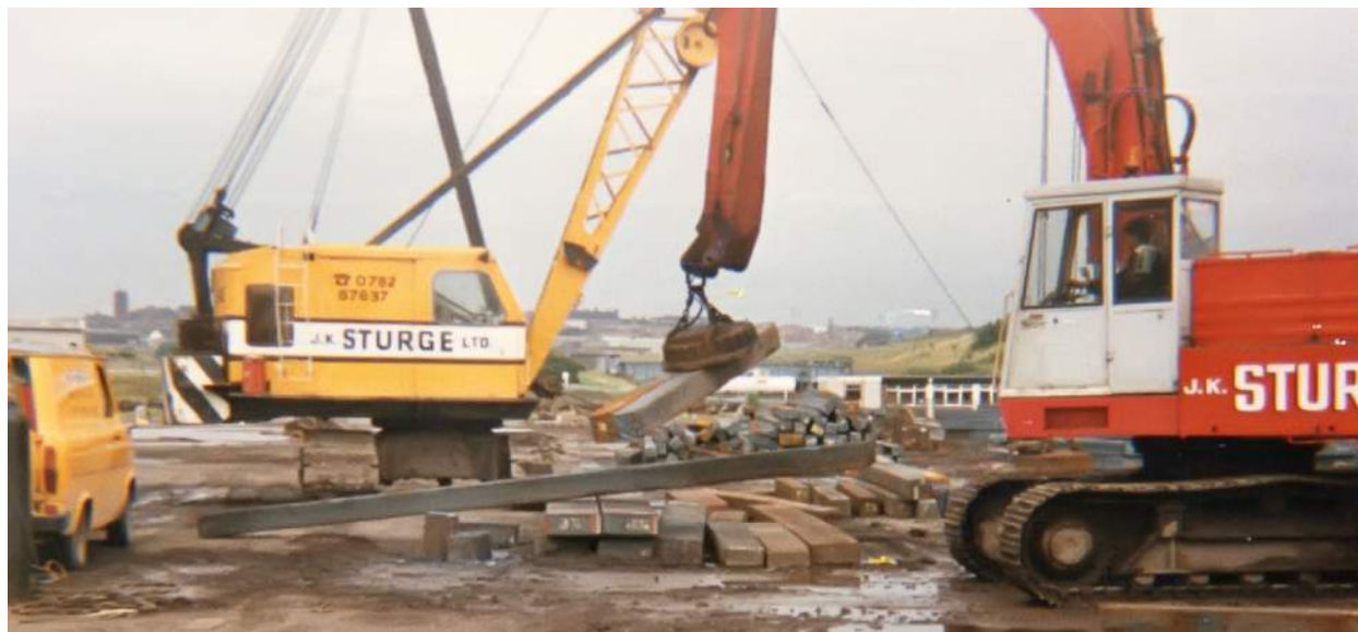
Figure 11.1 An industrial electromagnet is capable of lifting thousands of pounds of metallic waste. (credit: modification of work by “BedfordAI”/Flickr)
