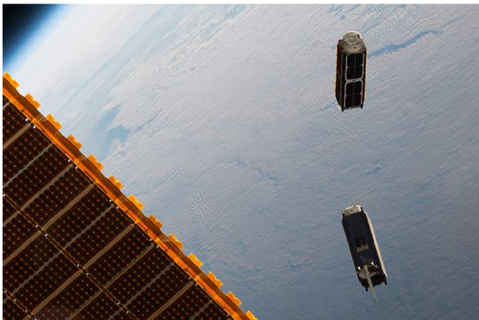
Figure 16.16 Two small CubeSat satellites deployed from the International Space Station in May, 2016. The solar sails open out when the CubeSats are far enough away from the Station. (credit: modification of work by NASA)
